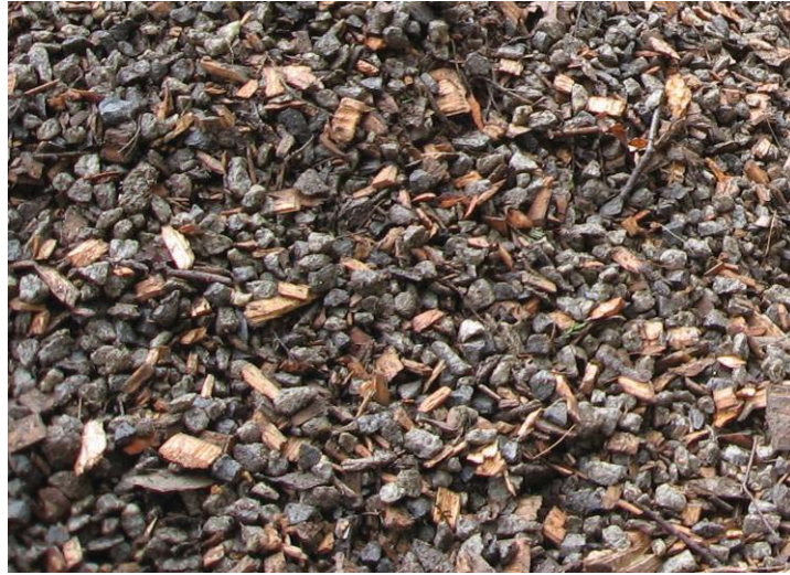
Figure 3: Inner Filter Core Comprised of 50% Wood Chips and 50% ½” Angular Stone
