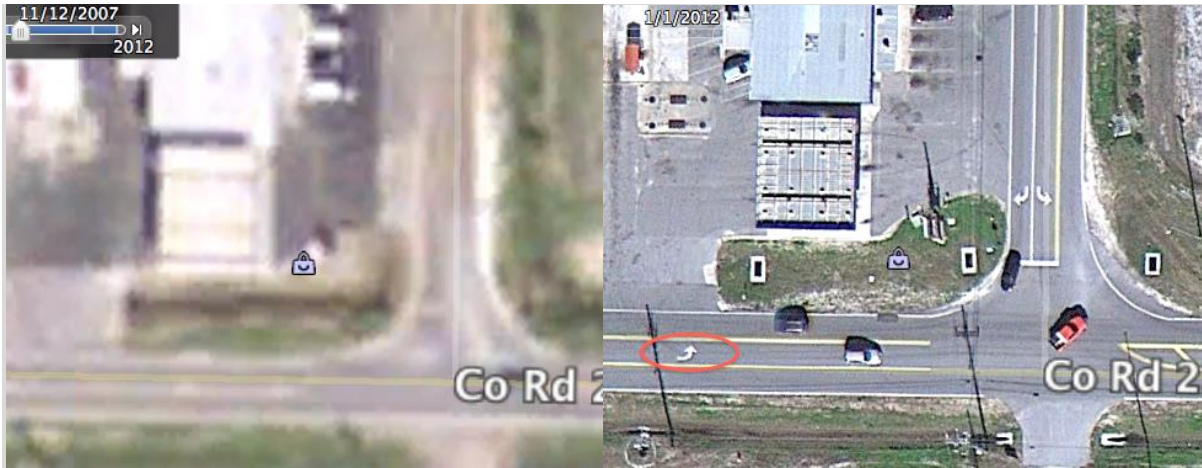
Figure 4-6: Example of Verifying Adding Left-Turn Lanes at Intersections Using Google Earth (Roadway ID: 46630000)
