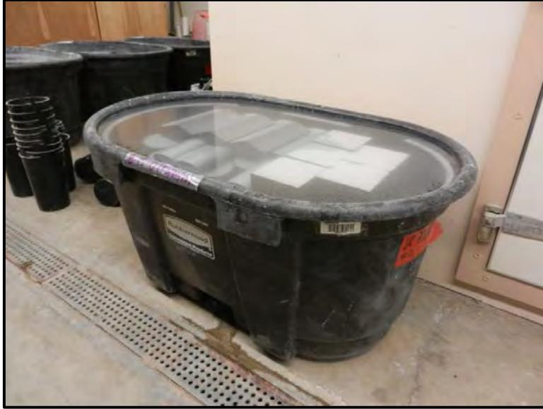
**Figure 3.3 Lime-Saturated Water Curing Tub**
