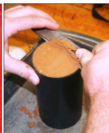
(f) Striking off Surface
