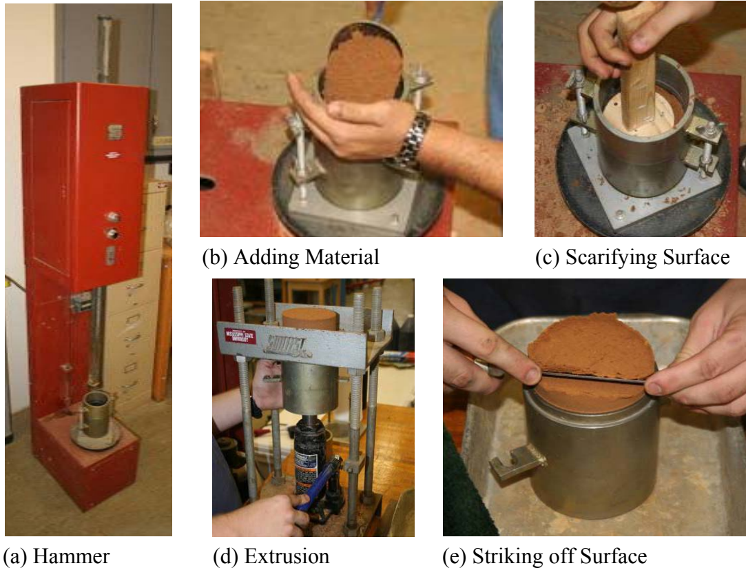
Figure 5.14. Example Proctor Compaction Photos
