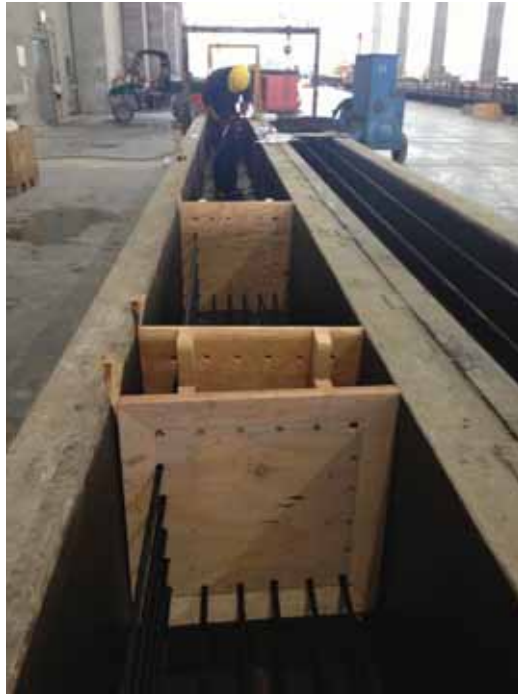
Figure H.3: View of precasting bed, showing wooden headers
