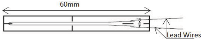
Figure 3.6: Strain gage schematic (Kyowa Strain Gage Manual)
