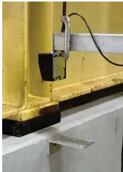
Figure 5.11: Laser device setup for measuring displacement
