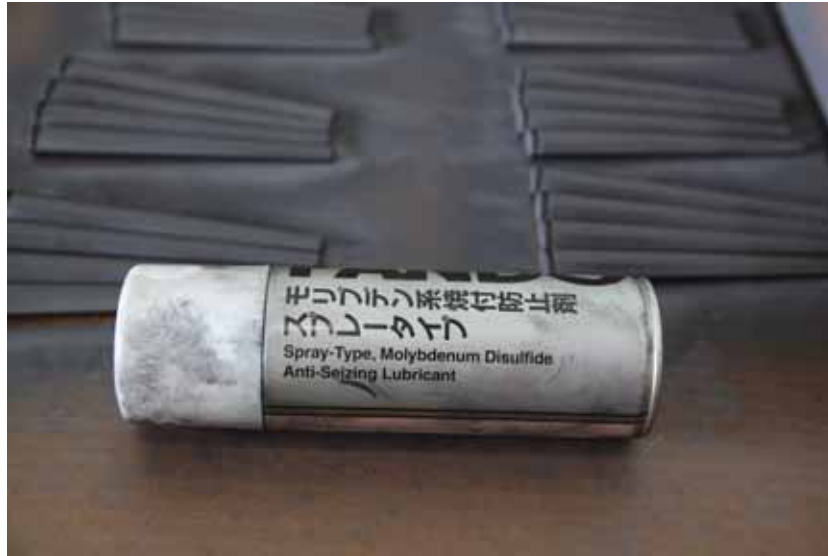
Figure H.7: CFCC wedges sprayed with Molybdenum Disulfide
