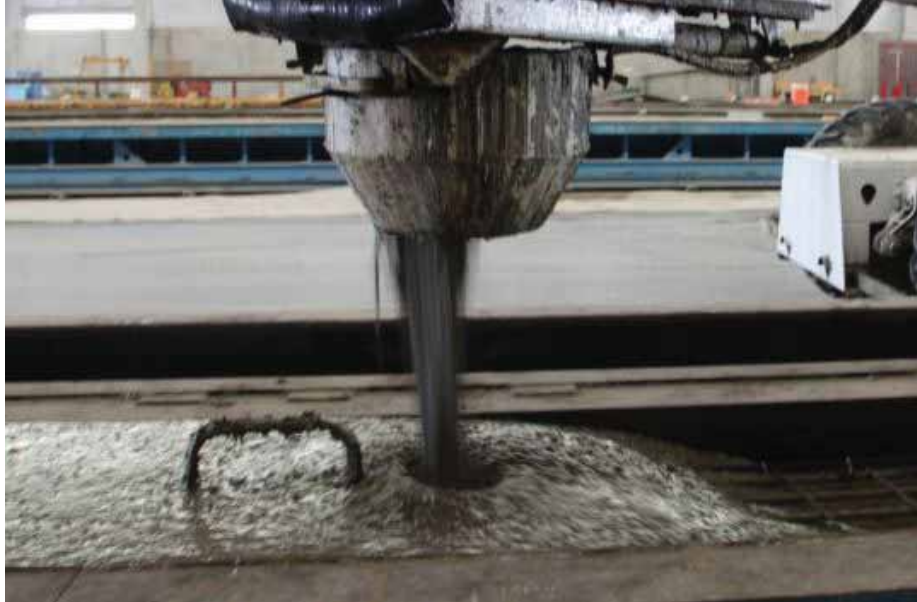
Figure 4.22: Casting using SCC
