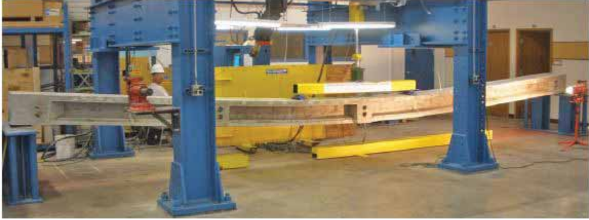
Figure 2.11: Load setup for decked bulb-T beams (Grace et al., 2012)
