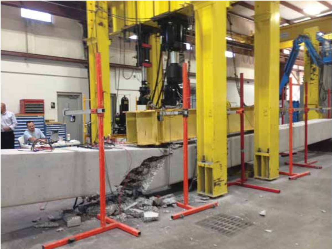
Figure 6.26: Failure under one of the load points
