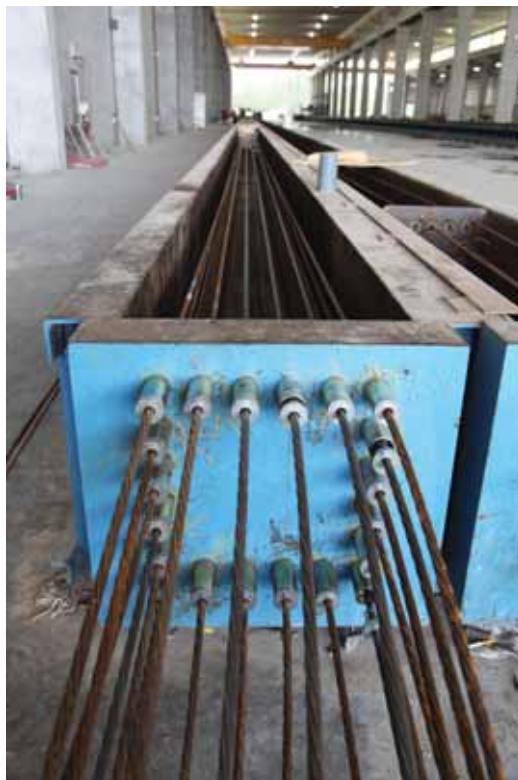
Figure H.21: Non-stressing end of self-stressing casting bed
