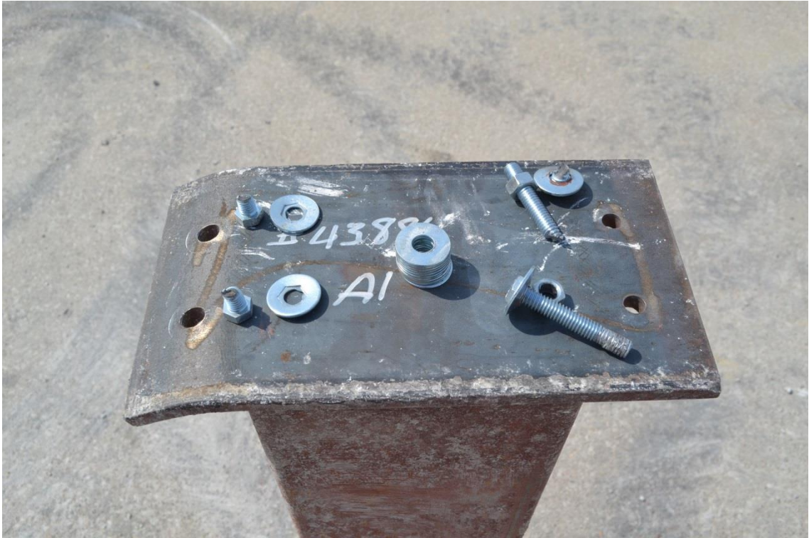
Figure 26. Bolts and Lower Base Plate, Test No. UBSPB-5
