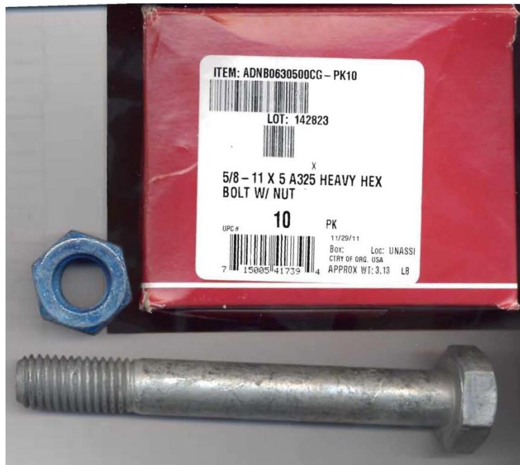
Figure A-18. 5/8-in. Dia. UNC Heavy Hex Nut, Test No. CP-1
