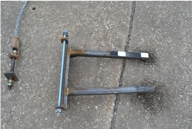
Figure 30. System Damage – Downstream Cable Anchor Bracket, Test No. HTCT-2
