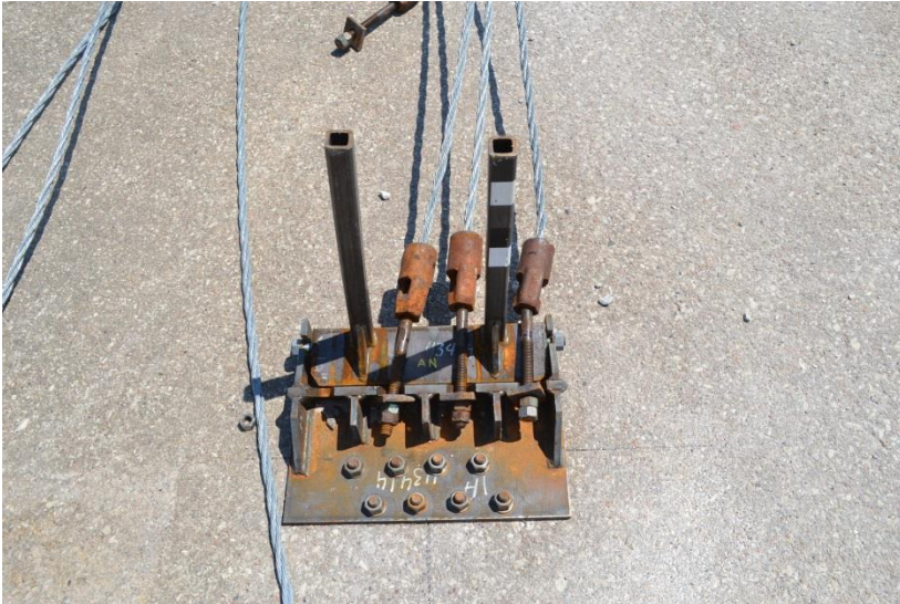
Figure 39. System Damage – Posts and Downstream Cable Anchor Bracket, Test No. HTCT-3
