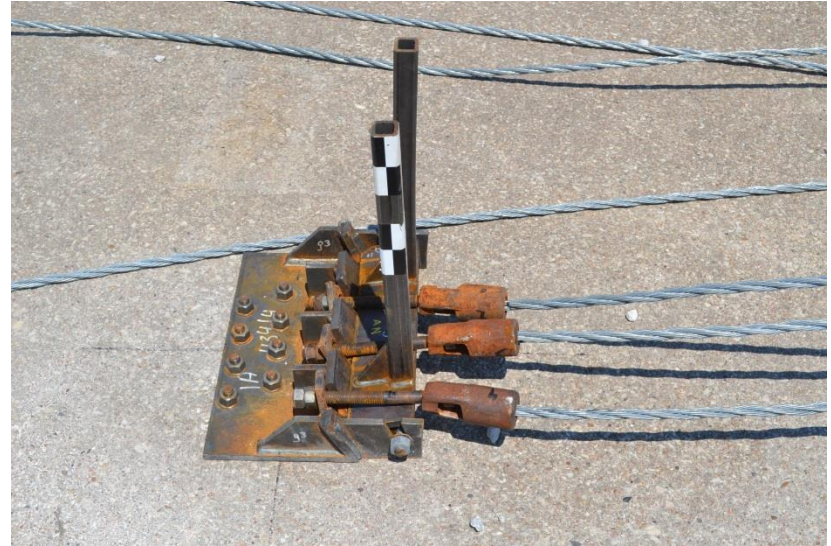
Figure 39. System Damage – Posts and Downstream Cable Anchor Bracket, Test No. HTCT-3
