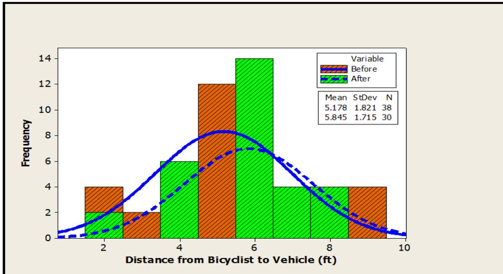
**FIGURE 6.3** Distribution of Bicyclist to Vehicle Separation: Riverside Drive
