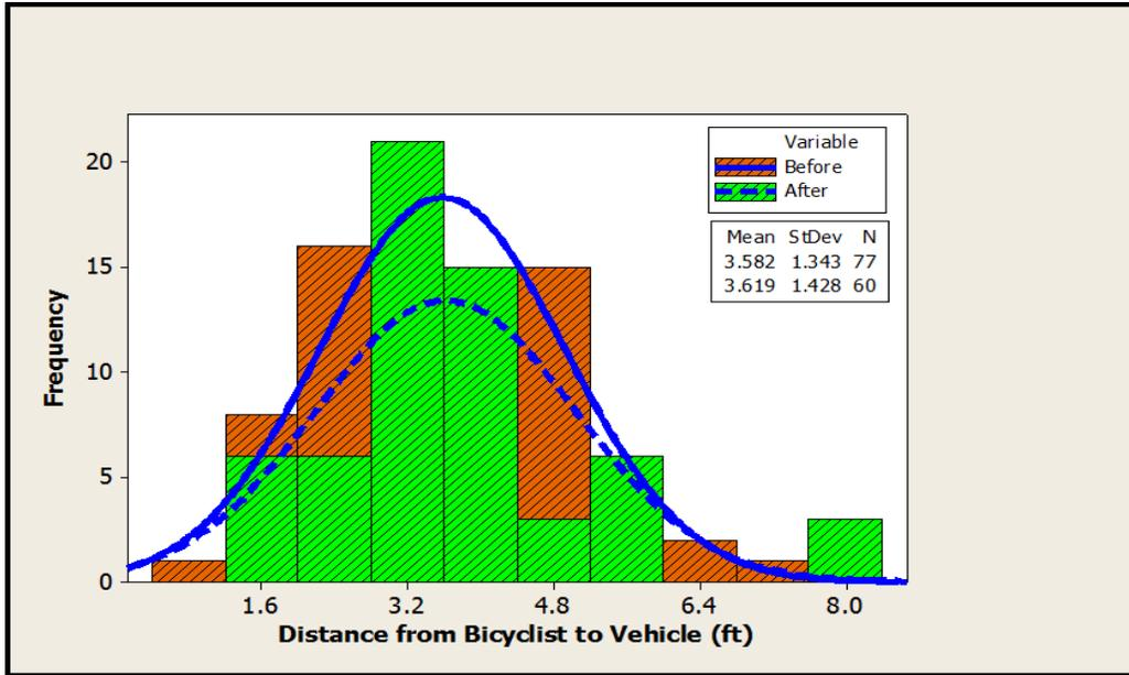
**FIGURE 6.6 Distribution of Bicyclist to Vehicle Separation: Bridge of Lions**
