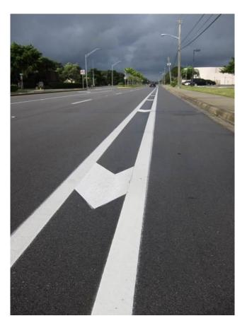
FIGURE 6.19 Section with 4-foot Bike Lane and 2-foot Buffer: Bailey Rd.
