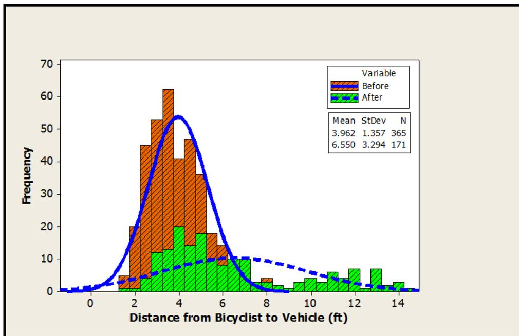
**FIGURE 6.9 Distribution of Bicyclist to Vehicle Separation: N 56<sup>th</sup> Street (Site A) Wider Outside Lane with Shared Lane Markings**
