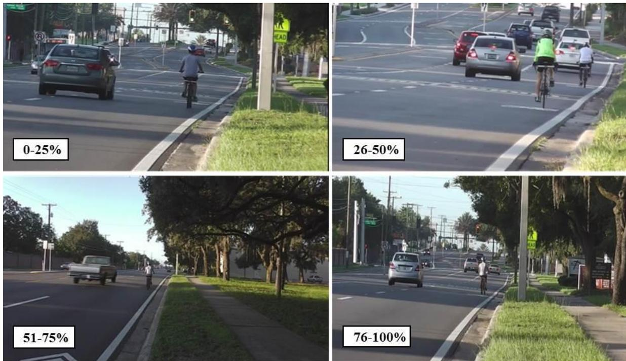
**FIGURE 5.2 Vehicle Lateral Shift into Adjacent Lane Quartiles**
