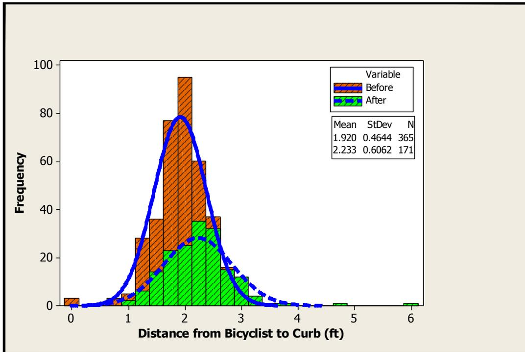
**FIGURE 6.10 Distribution of Bicyclist to Curb Distance: N 56<sup>th</sup> Street (Site A) Wider Outside Lane with Shared Lane Markings**
