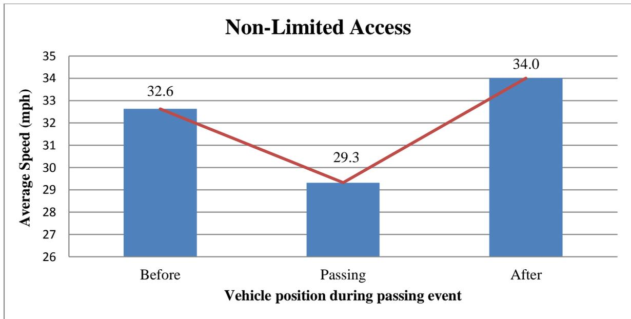
**FIGURE 6.31 Average Vehicle Speed during Passing Events (Non-Limited Access Sites)**
