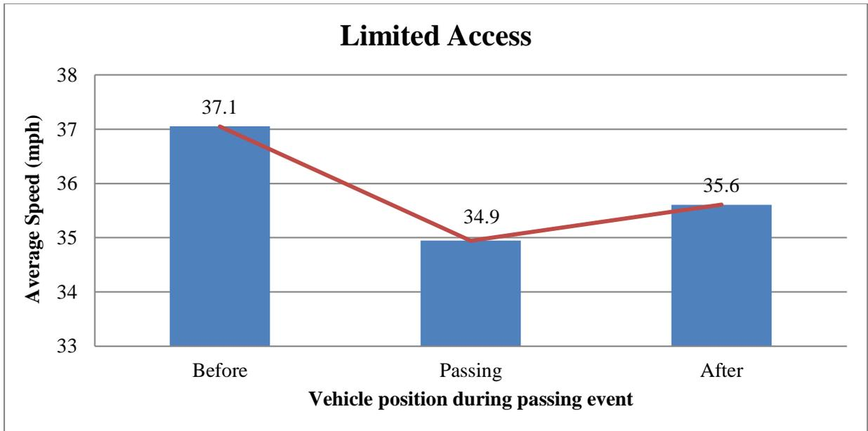
**FIGURE 6.32 Average Vehicle Speed during Passing Events (Limited Access Sites)**
