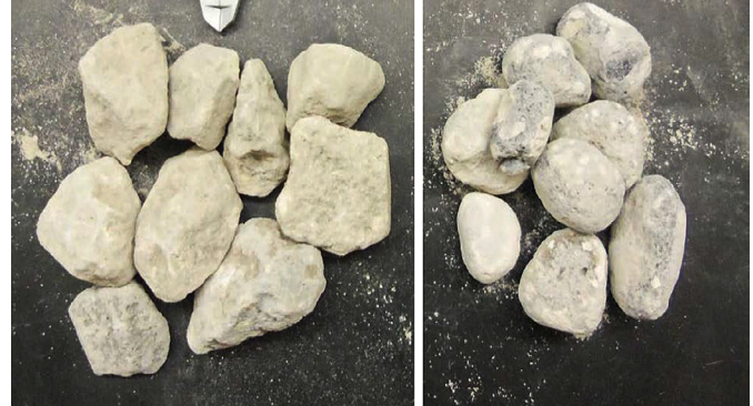
RCA before (left) and after (right) standard abrasion testing. The rounding and general loss of size shows significant susceptibility to abrasion.
