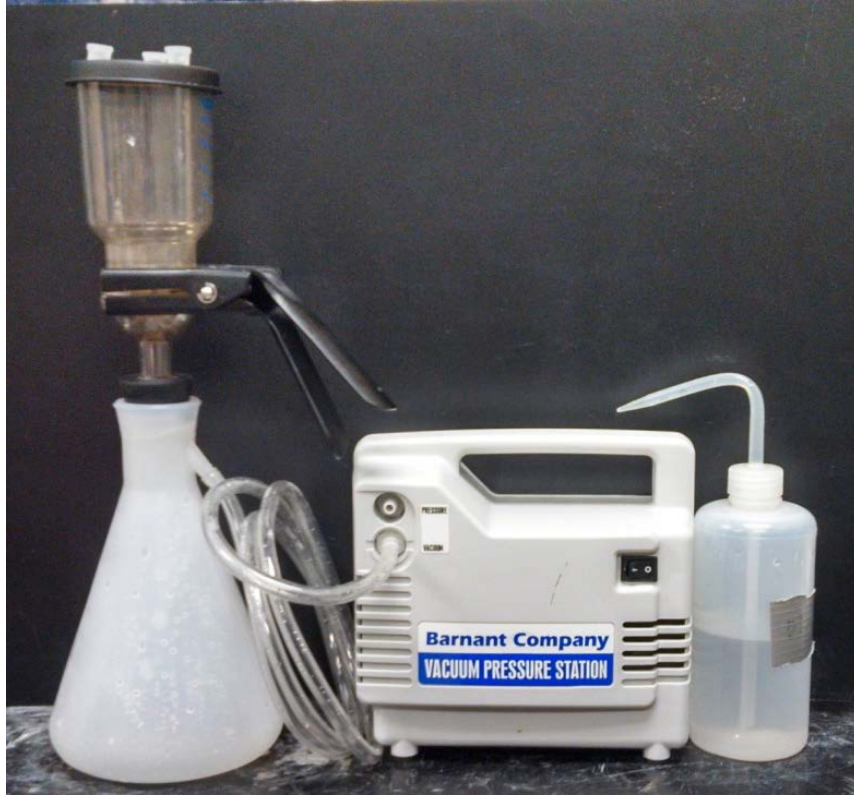
Figure 6.9: Filtration Equipment Required for ASTM D5907
