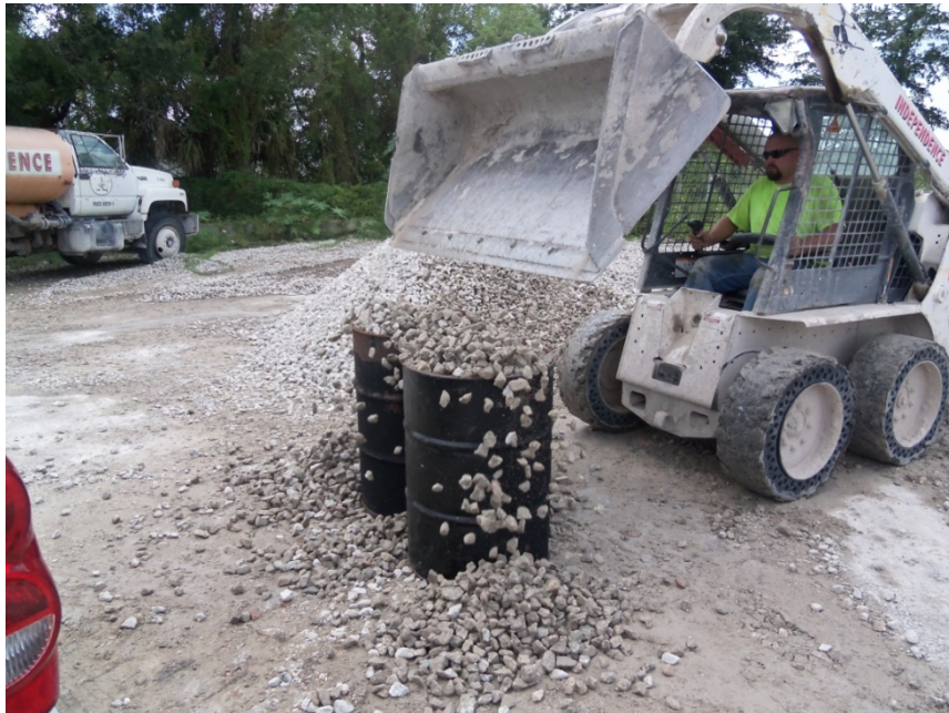
Figure 3.1: RCA Being Obtained from an Orlando, FL Recycling Facility
