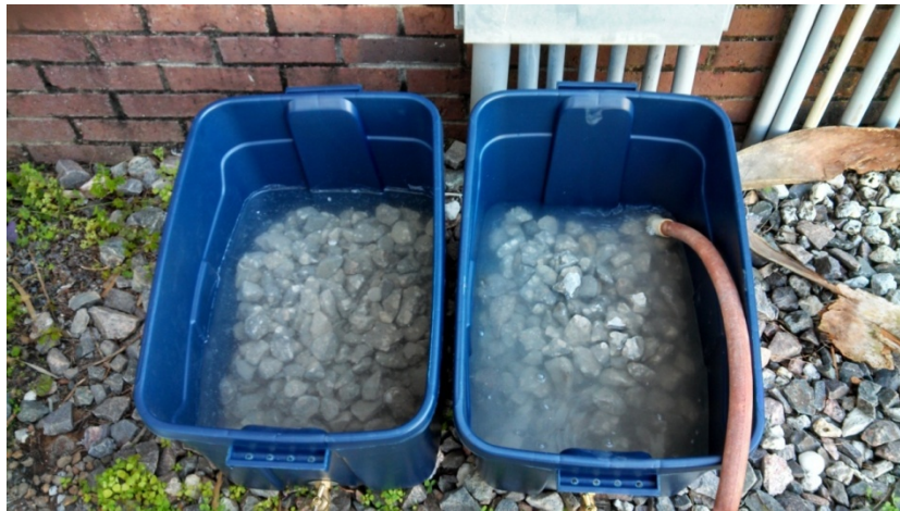
Figure 3.9: Aggregate Washing Setup
