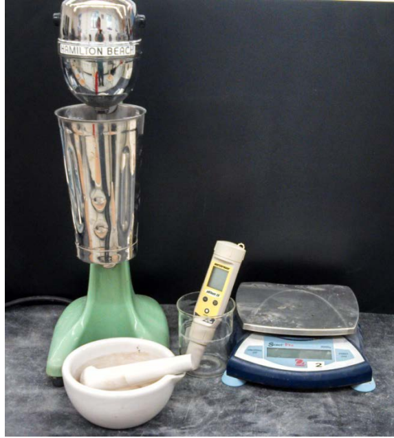
Figure 4.2: pH Testing Setup
