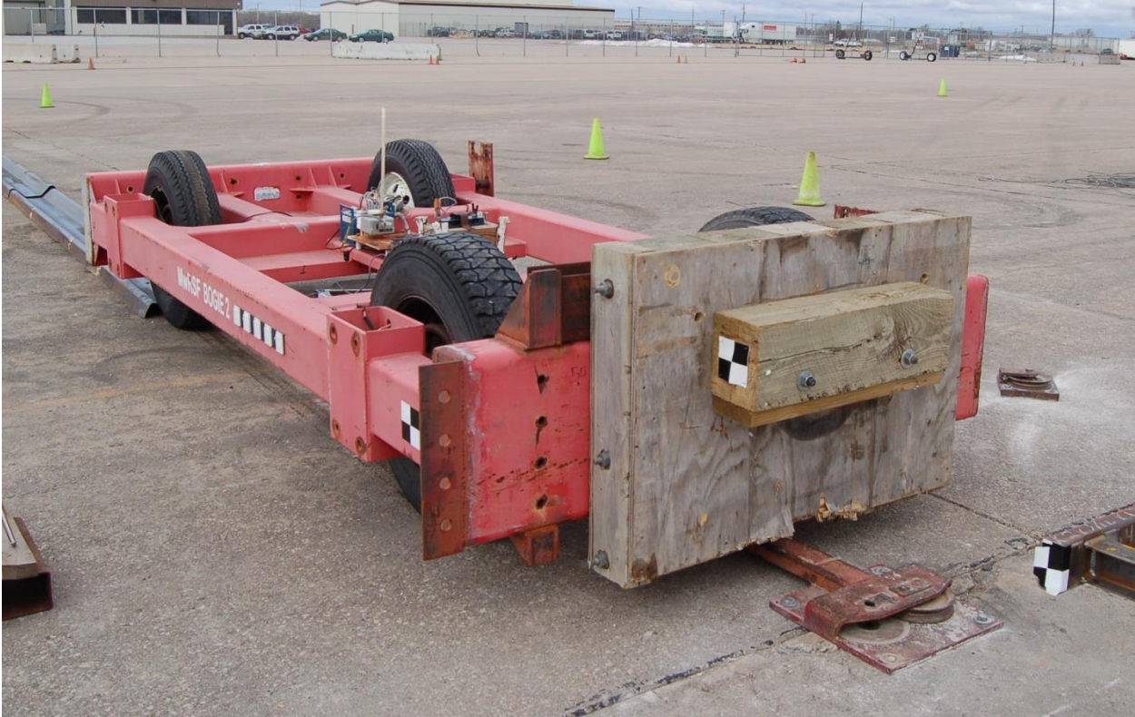
Figure 3. Rigid-Frame Bogie on Guidance Track, Test No. HSF14-5
