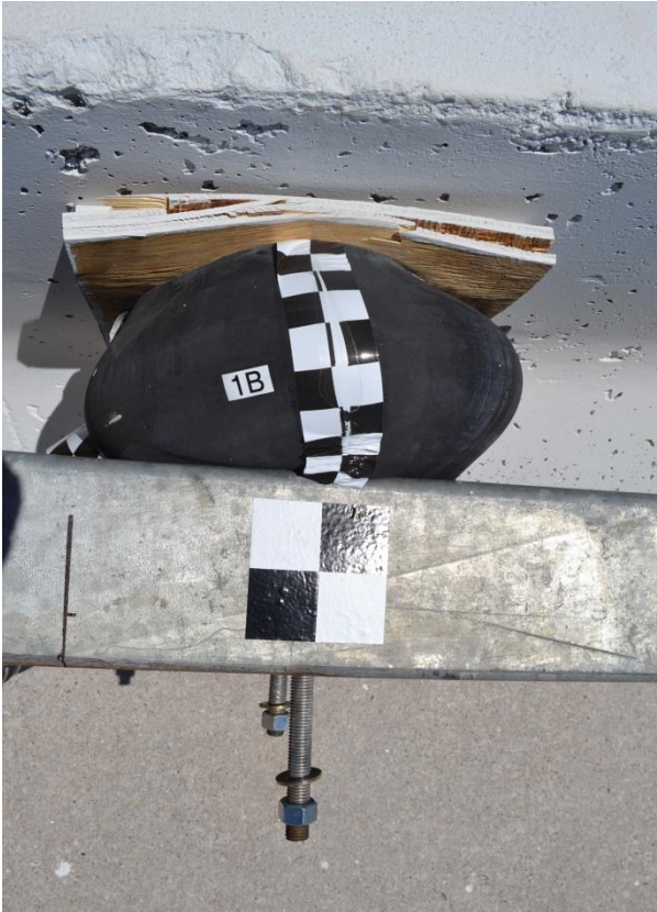
Figure 66. Cylinders Post-Impact Damage, Test No. SFHC-1
