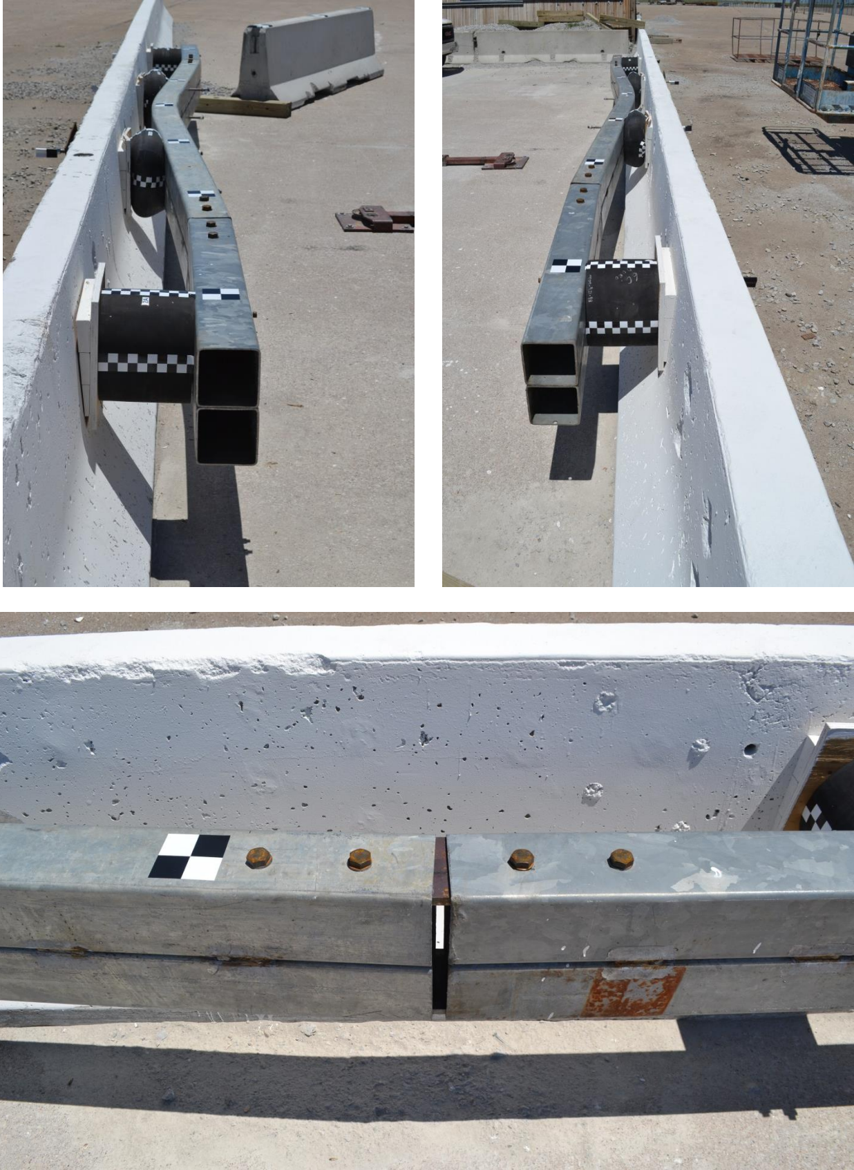
Figure 67. Post-Impact Damage, Test No. SFHC-1
