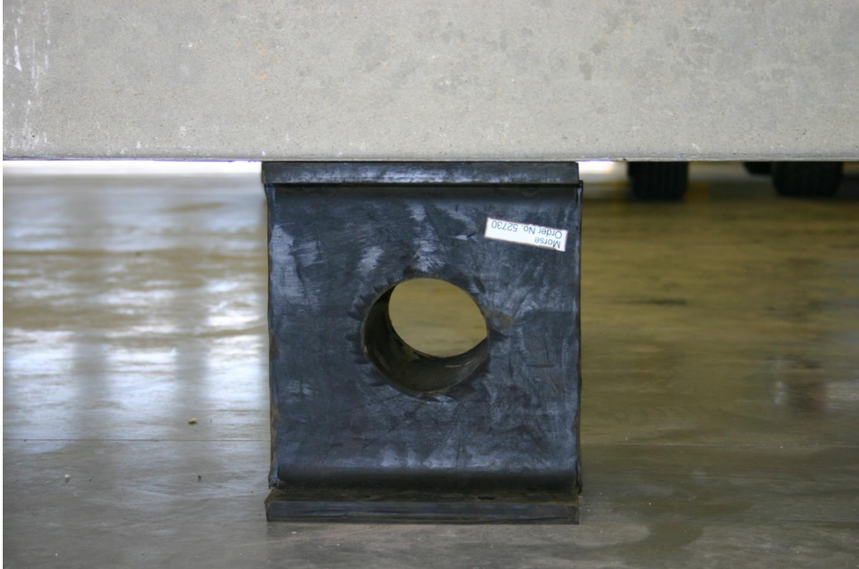
Figure 97. System Deflection at 7,000-lb (3,175-kg) Load, Test No. SFHS-7
