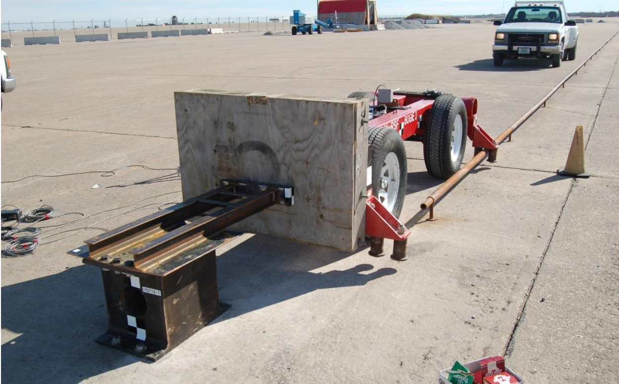
Figure 38. Bogie Setup, Test Nos. HSF14-2 through HSF14-4
