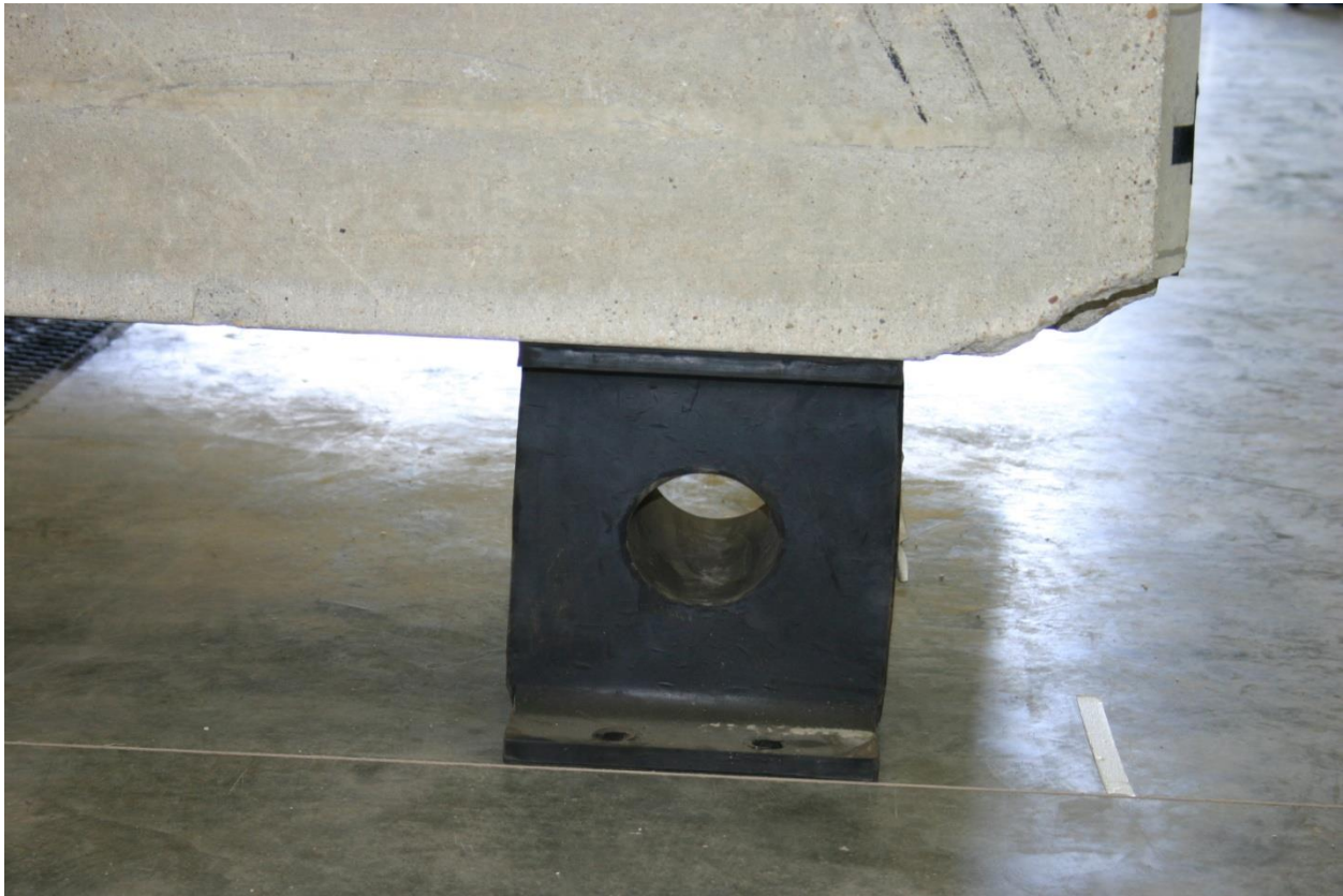
Figure 101. System Deflection at 4,994-lb (2,265-kg) Load, Test No. SFHS-10
