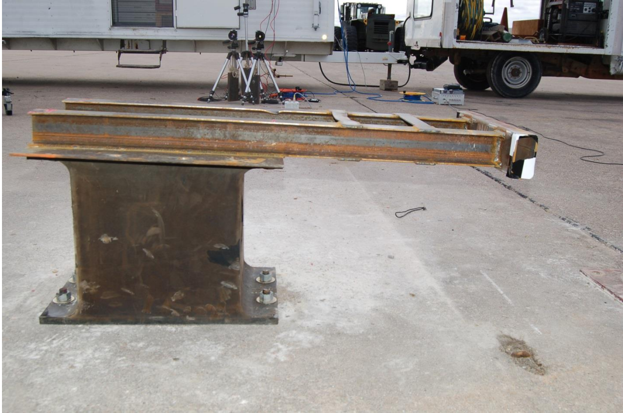
Figure 50. Post-Impact Damage, Test No. HSF14-5
