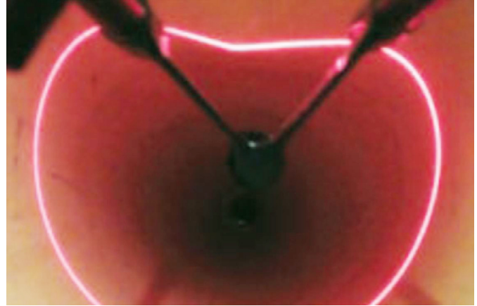
One type of laser profiling projects a ring of light onto the interior of a pipe. Notice the depression at the top of what was originally a perfectly round pipe.
