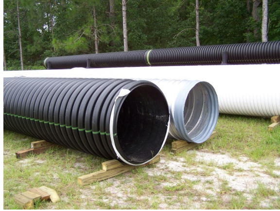
Figure 3-9: Positioned PVC, CMP, and HDPE Pipes
