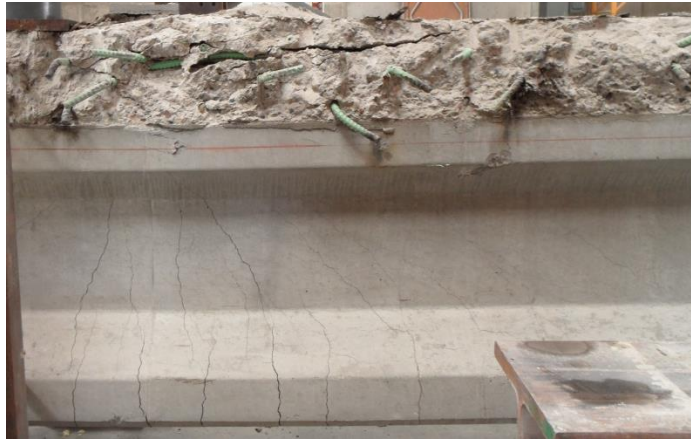
Fig. 5.11 G4-2d(b) (bottom) and ANSYS 2d test (top) failure cracking
