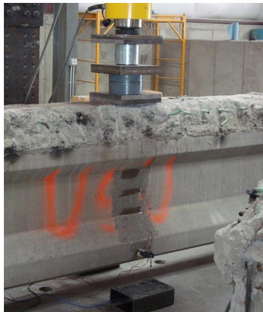
Fig. 4.6 mid-span test set up in lab
