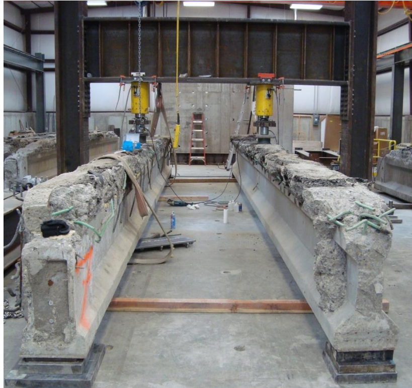
Fig. 4.1 Reaction frame with two girders ready to test.
