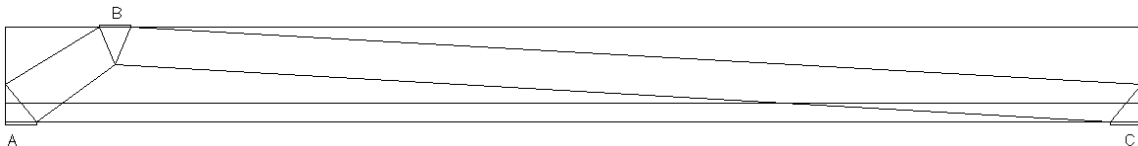
Fig. 5.1 Strut and Tie model of the girder with compressive struts AB and BC and tie AC
