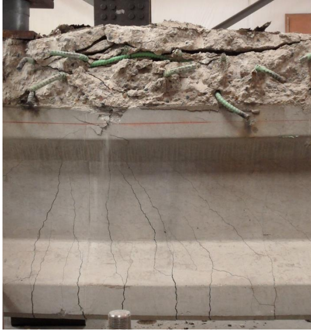
Fig. 4.20 G4-2d(b) just prior to failure
