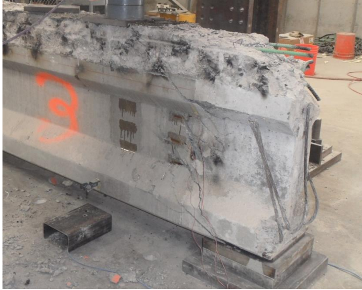
Fig. 4.16 Failure crack of G3-1d(a)
