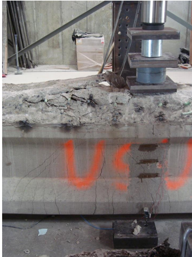
Fig. 4.7 Cracking prior to failure of mid-span test
