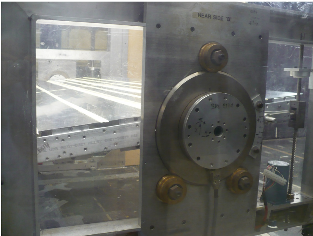
FIGURE 1.10 STATIC SECTION MODEL TEST RIG
