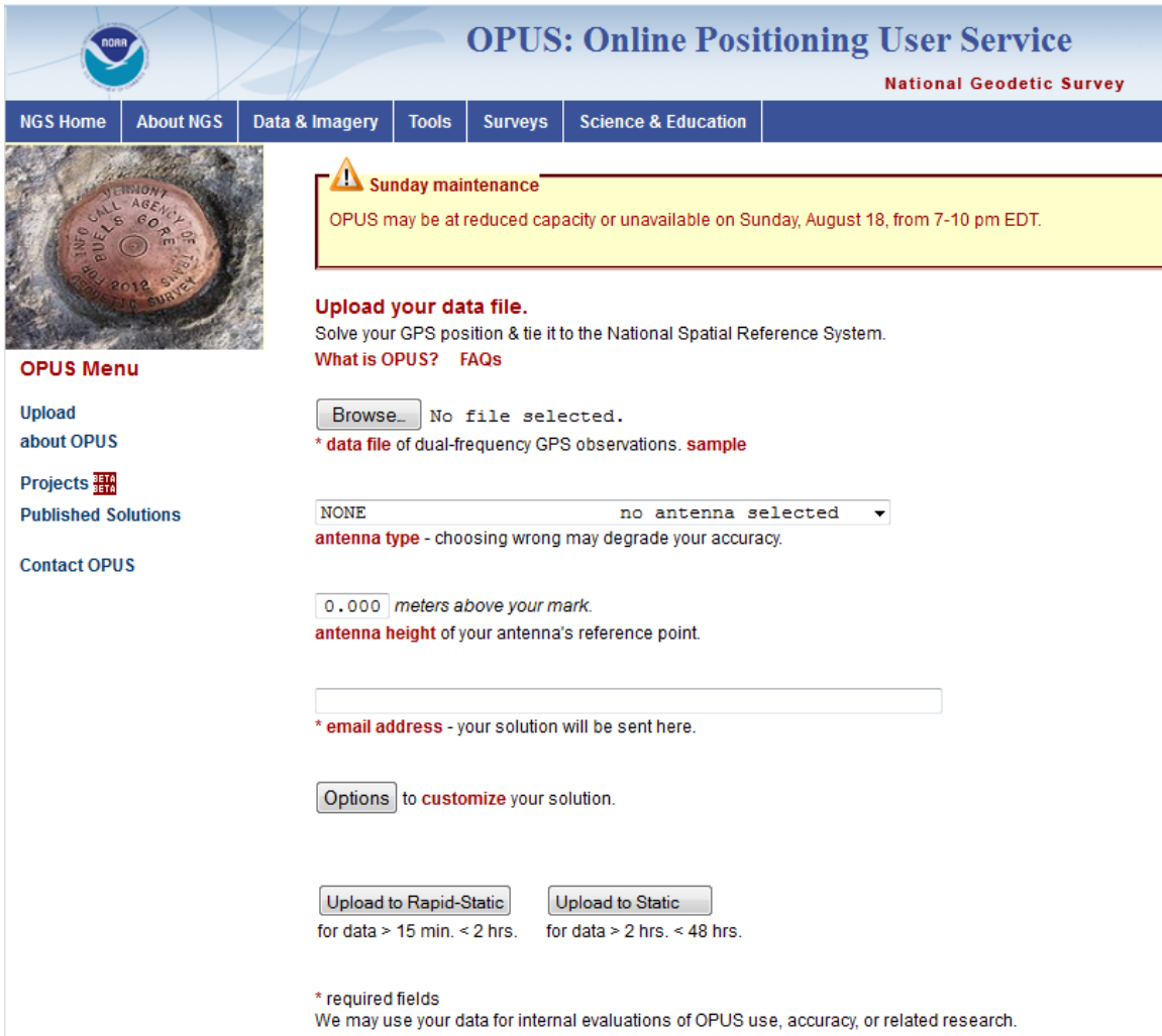
Figure 4-1 - The NGS's Online User Positioning Service (OPUS) web application used for submitting static GPS observation files to OPUS for processing
