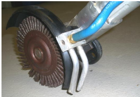
Figure 2.2 Behind wheel air nozzle
