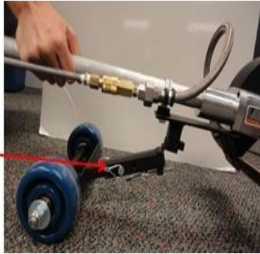
(a) 2 nd Generation : foldable wheel assembly
