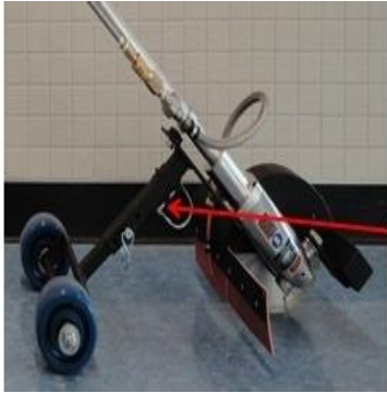
(a) 2 nd Generation : foldable wheel assembly
