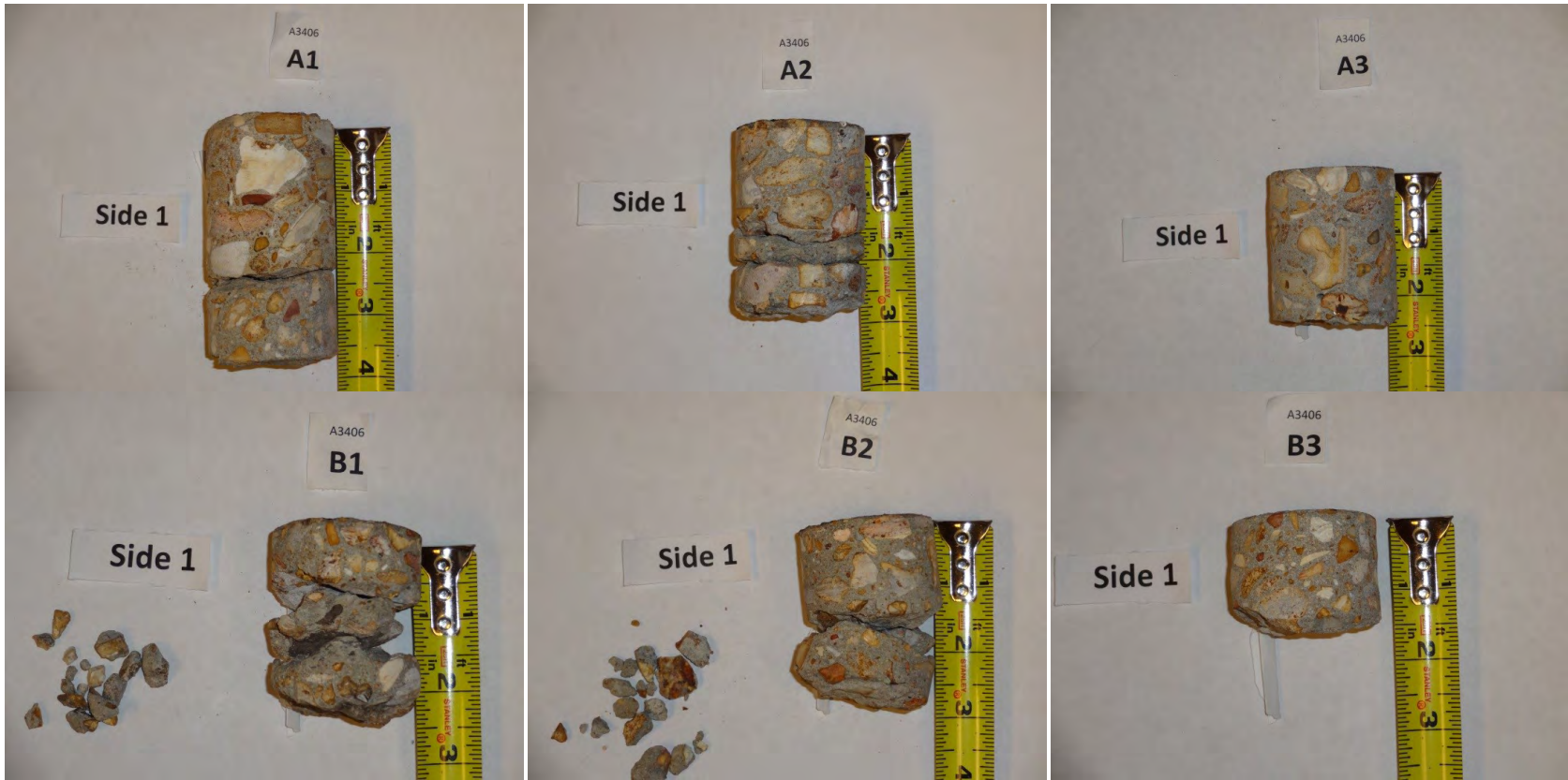
Figure 4-20 Cores Extracted From Bridge A3406
