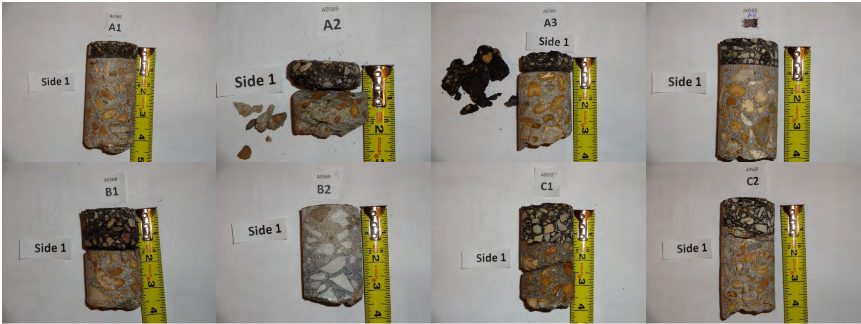
Figure 4-2 Cores Extracted From Bridge A0569
