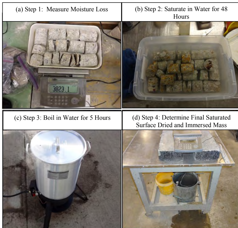
Figure 4-1 Process of Determining Volume of Permeable Pores
