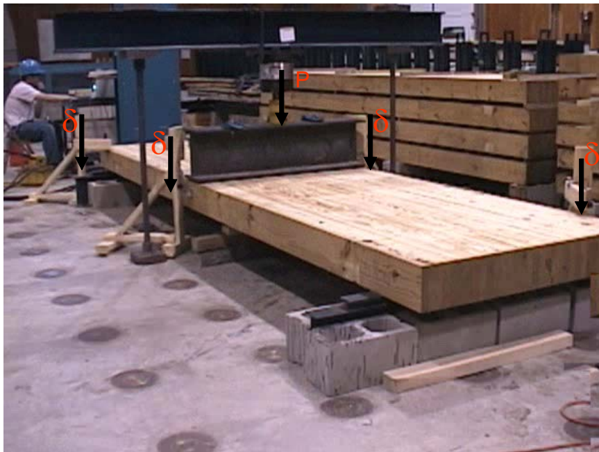
Figure 3. MOE Test Schematic
