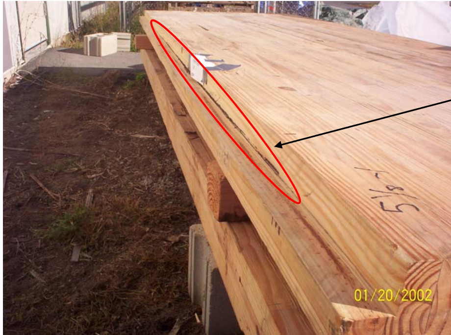
Figure 11a. Intial Failure - Tension Perp at Tongue/Panel Interface
