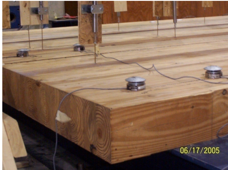
Figure 8. Compression Washers Used to Monitor Bolt Forces
