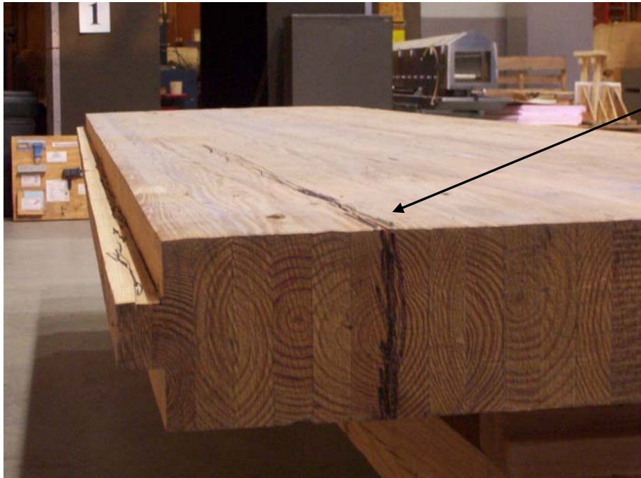
Figure 13a. Shear Out Failure of Tongue Panel
