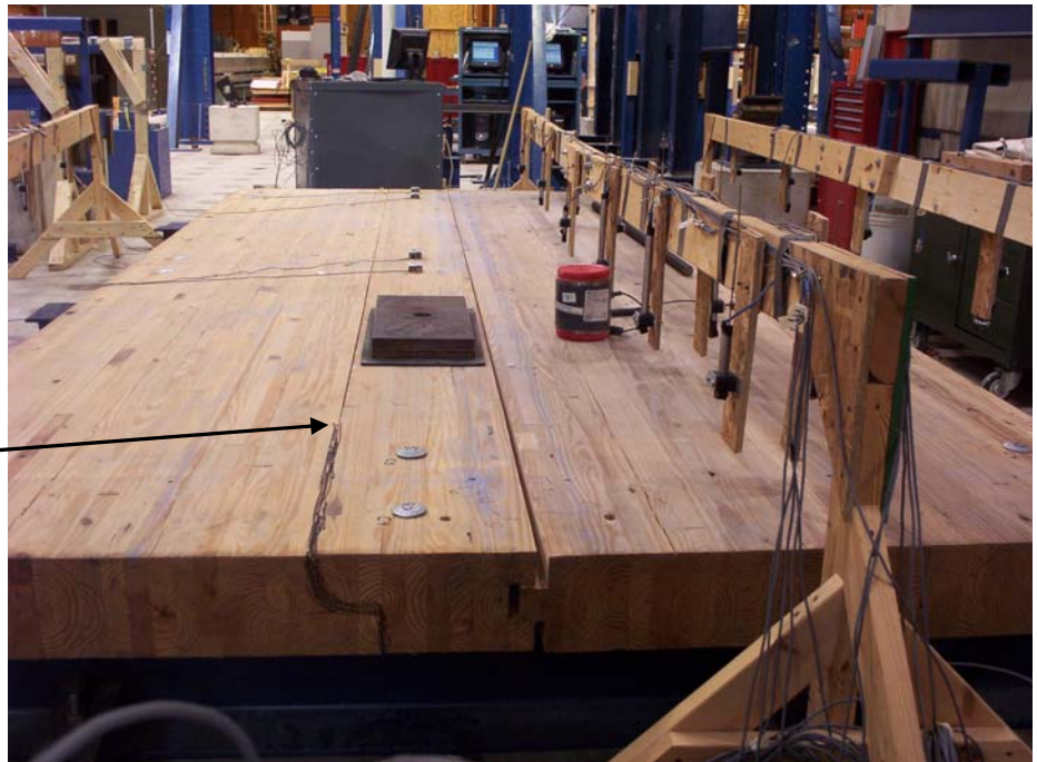
Figure 13b. Shear Out Failure of Groove Panel
