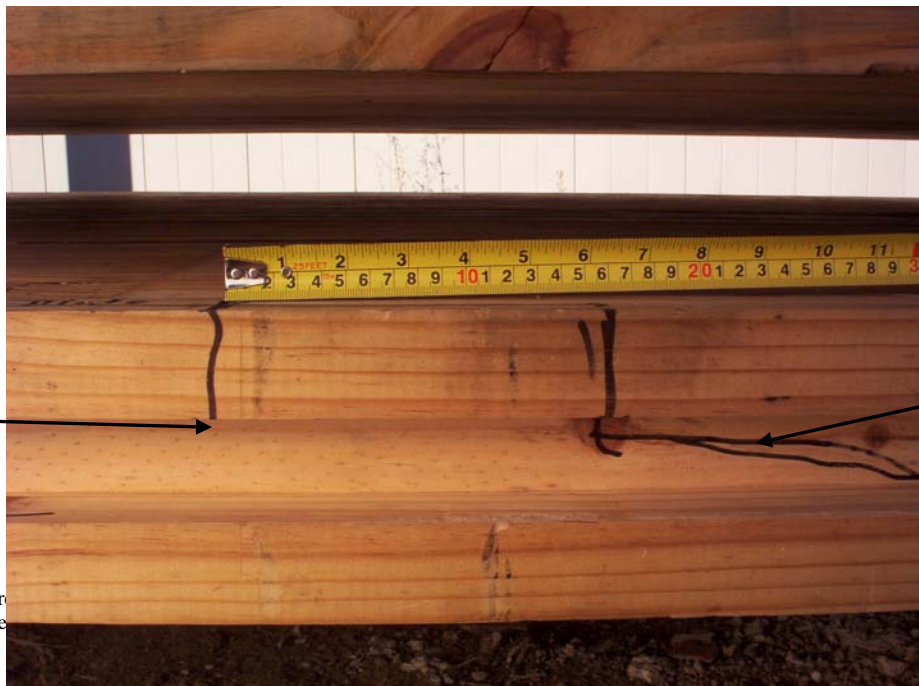
Figure 11b. Secondary Failure – Localized Shear Failure Near Load Patch
