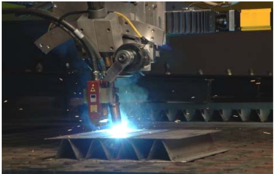
Figure 1.3 Hybrid Laser Welding on Sandwich Panel (Abbot et al. 2008)
