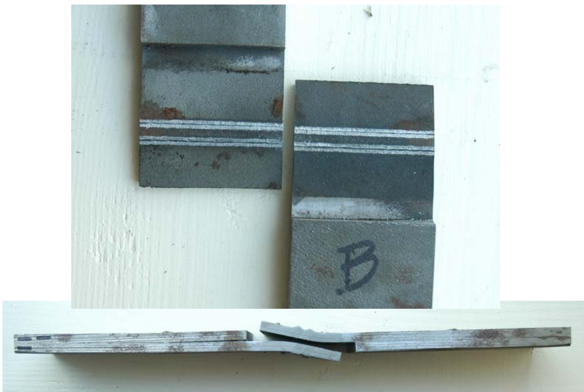
Figure 3.13 Typical Failure in SWT-4W Specimen
