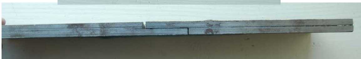
Figure 3.15 Typical Failure in SWL-4W Specimen
