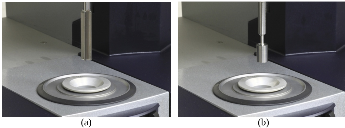
Figure 22 – Possible Alternate DSR Geometries for Measuring High Temperature Properties of CRM Asphalt Binders; (a) Couette & Bob and (b) Vane & Couette
