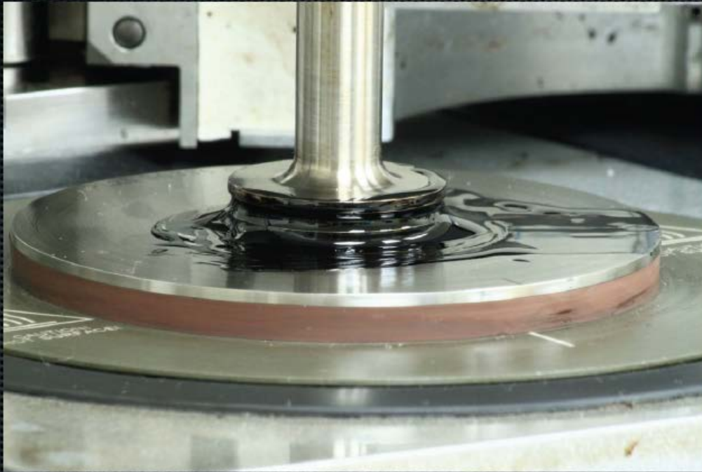
Figure 18 – 2.0mm Gap Height Immediately After Testing at 88°C
