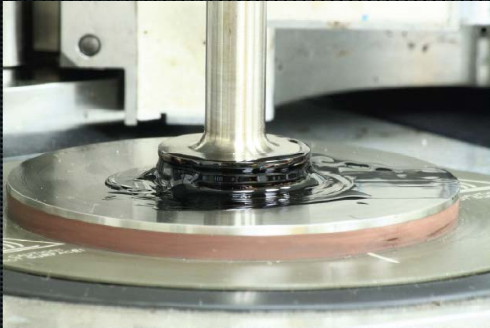
Figure 17 – 2.0mm Gap Height Immediately After Testing at 82°C
