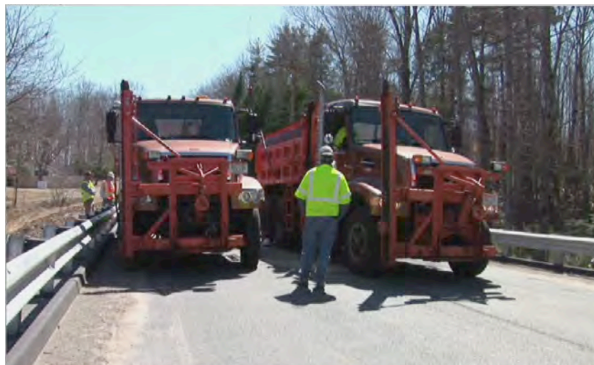
Figure 6: Trucks Used in Testing of Neal Bridge
