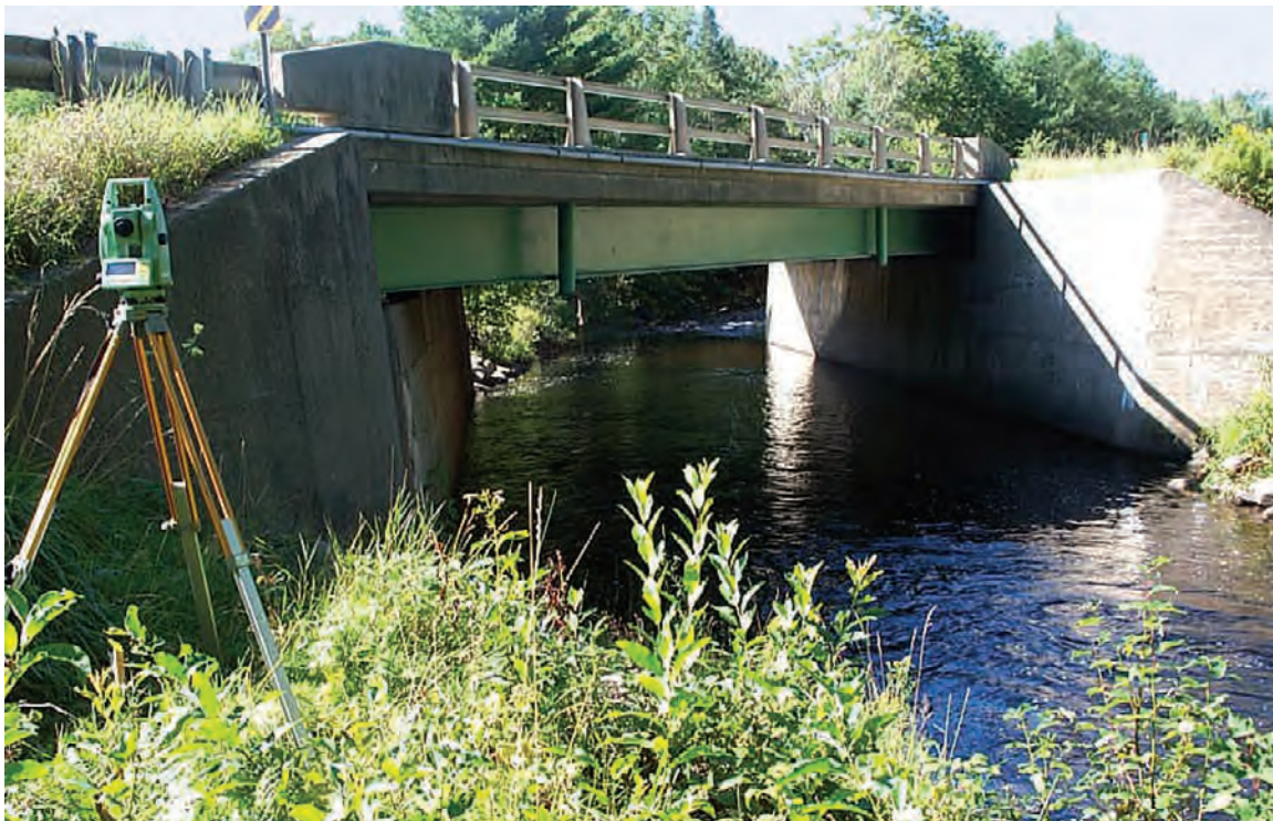
Figure 2. Total station theodolite used to collect survey data at the East Branch of the Wesserunsett Stream at Athens, Maine, August 25, 2004.
