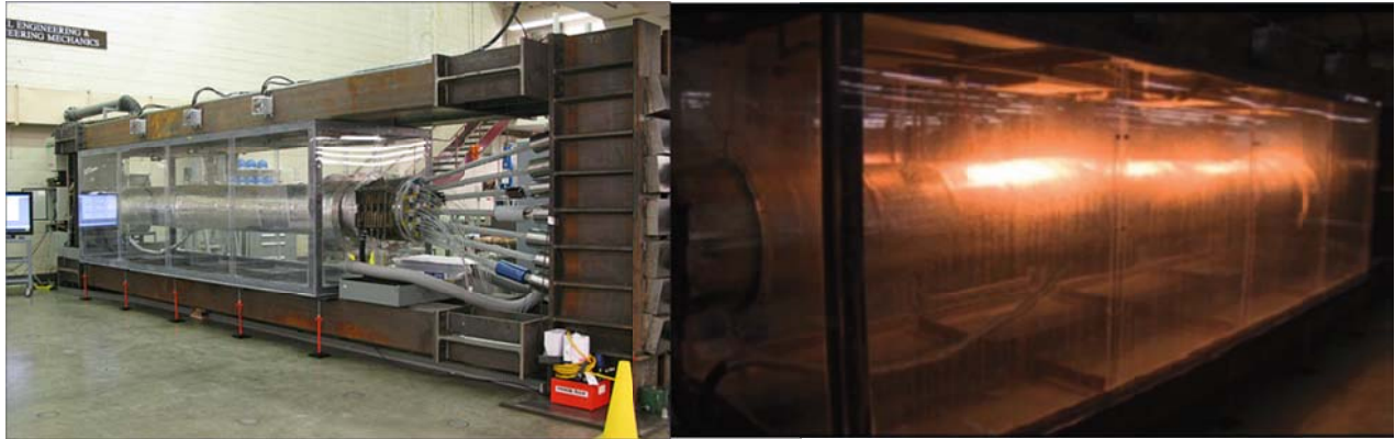
Figure 15: Mock-up cable specimen and environmental corrosion chamber; Left: angled view of specimen [Khazem, Serzan & Betti, 2012] & Right: heating phase of cyclic environmental conditions [Sloane et al., 2012]
