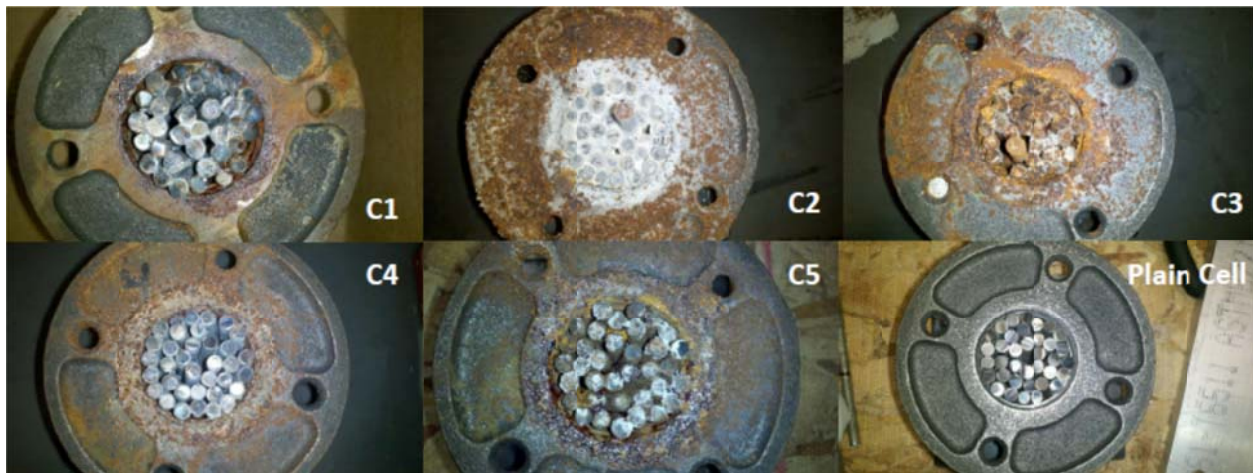
Figure 6: Visual of cumulative corrosion for each cell after completion of laboratory testing
