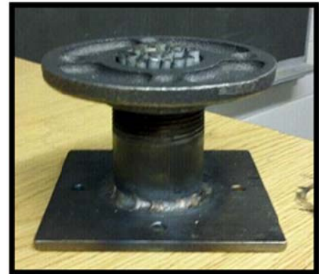
Figure 4: Corrosion cell with wires
