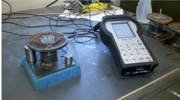
Figure 5: Set-up for laboratory corrosion cell testing
