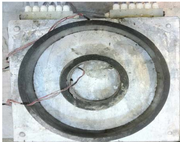
Figure 7.3: Dual ring test used to monitor stresses while creating restrained boundary conditions for the concrete
