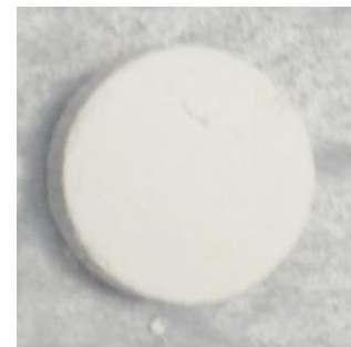
Figure 6. An MgTiO 3 pellet as printed using an ExOne X1-Lab model powder bed printer.
