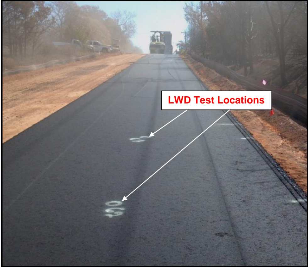
Figure 3. Representative LWD test locations at Apple Valley Road Project in Edmond, OK.
