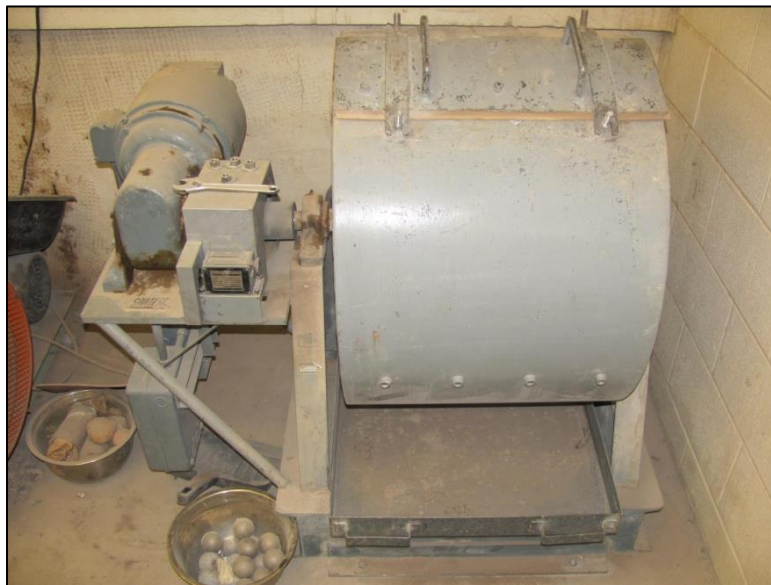
Figure 5.3 Apparatus Used for L.A. abrasion Test.
