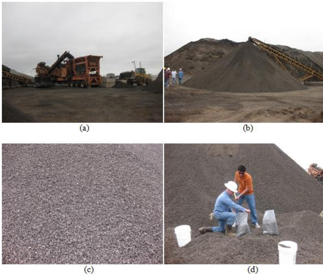
Figure 3.1 (a) Processing of RAP1 millings, (b) Stockpile of RAP1 millings, (c) Close view of I-35 (RAP1) millings, and (d) Collection of I-35 (RAP1) millings
