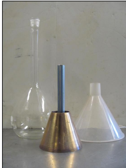
Figure 5.2 Apparatus Used for determination of Specific Gravity of Fine Aggregates.
