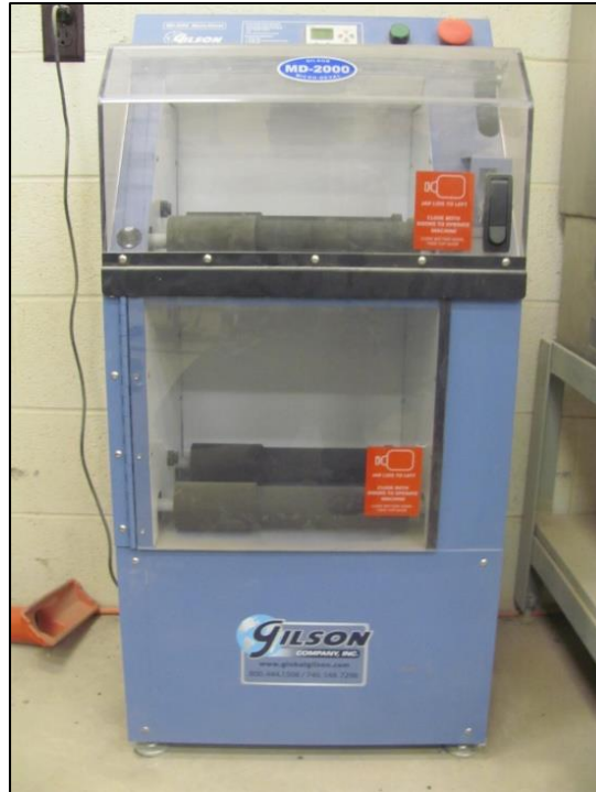
Figure 5.4 Apparatus Used for Micro-Deval Test.
