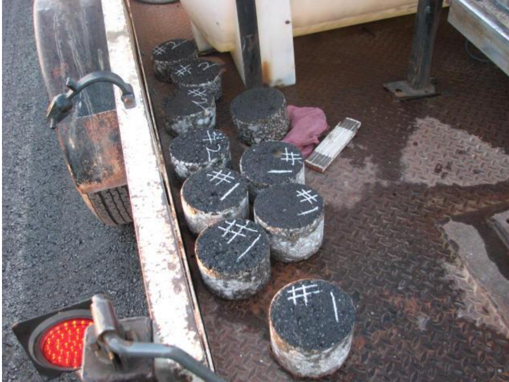
Figure 3.25 Obtained Cores from S3 Layer for Test Site 2.
