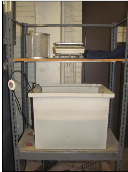
Figure 5.1 Apparatus Used for determination of Specific Gravity of Coarse Aggregates.
