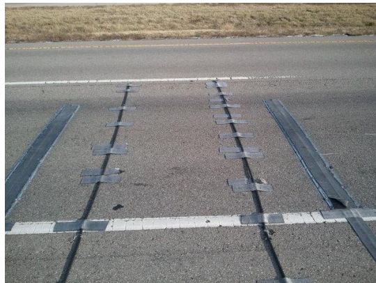
Figure 4. 5. Piezoelectric sensors and full length of the fixture covered most of the lane area
