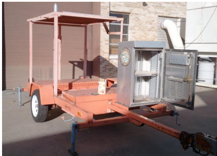
Figure 2. 8. Portable WIM trailer before the installation of the power system, WIM controller and the REECE
