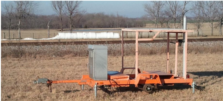
Figure 4. 4. The portable WIM trailer deployed in Wagner
