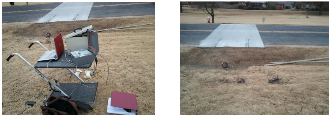
Figure 2. 1. WIM controllers and sensor layout
