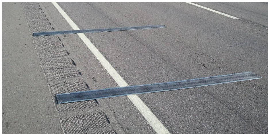
Figure 4. 6. The initial piezoelectric sensors in the second deployment
