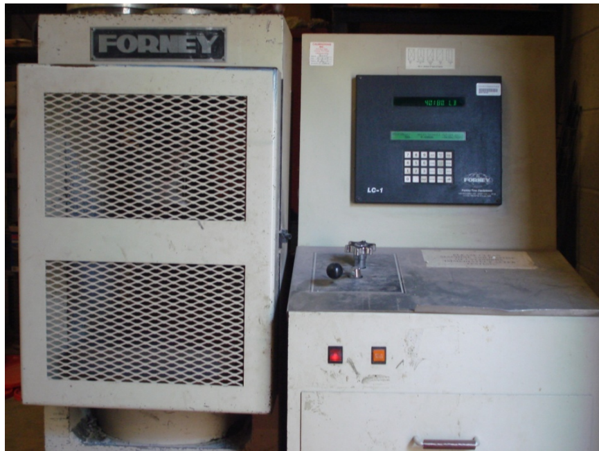
Figure 4.33: Forney Machine Used for Compression Strength Test
