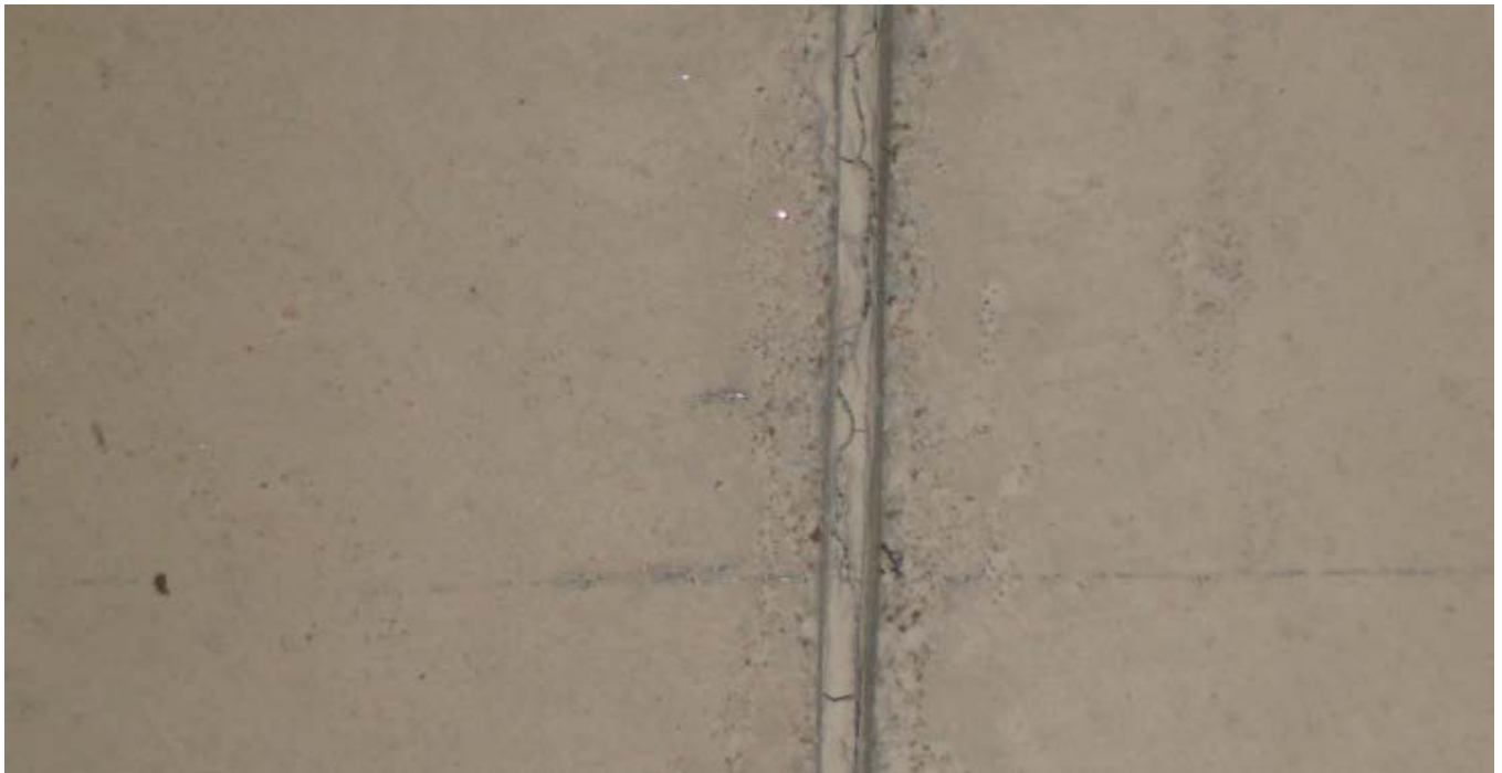
Figure 5.8: Top View of joint expansion or crack at large scale slab specimen
