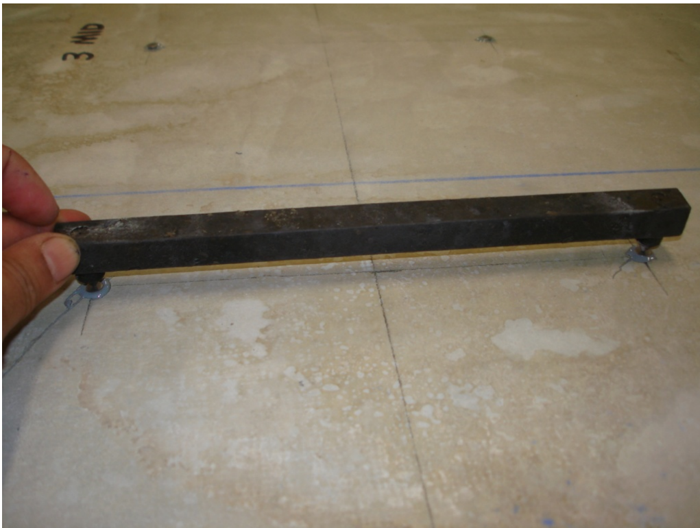
Figure 4.26: Fixing Demec Targets at Required Location
