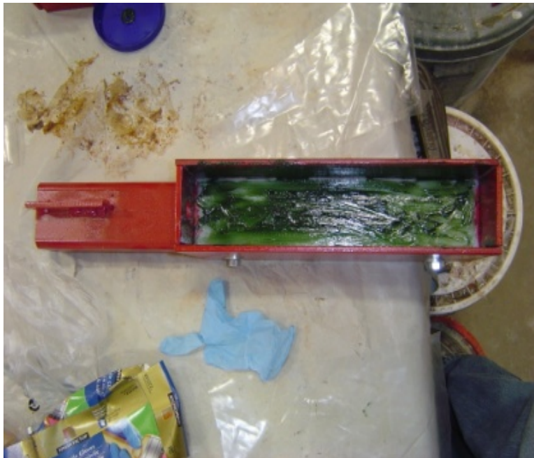
Figure 5.30: Grease layer applied over the steel walls and the Teflon bottom
