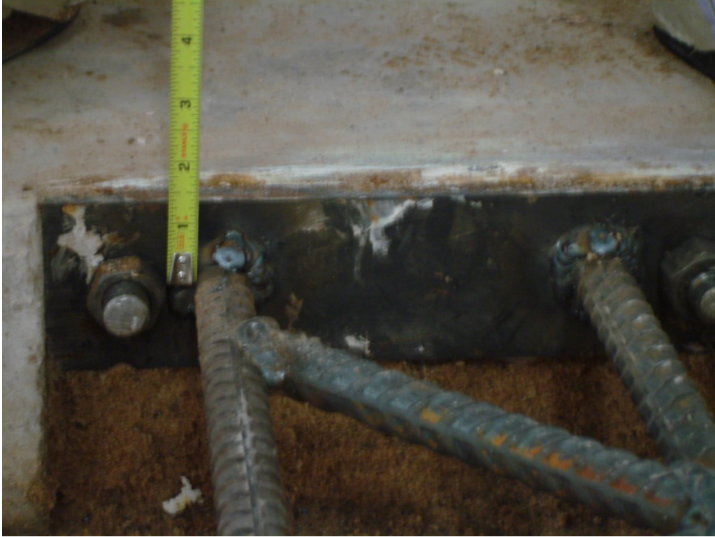
Figure 4.4: Welded Truss at Mid- Height of the Plates
