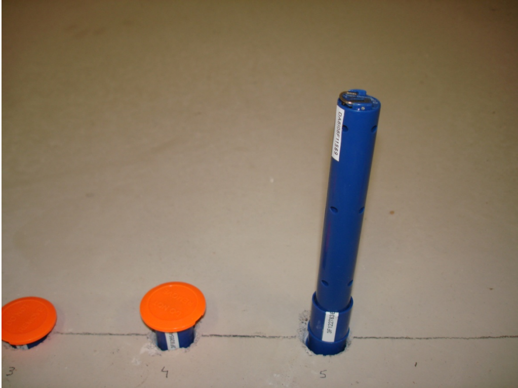
Figure 4.42: RH meter for Measuring Temperature and Moisture of the Slab
