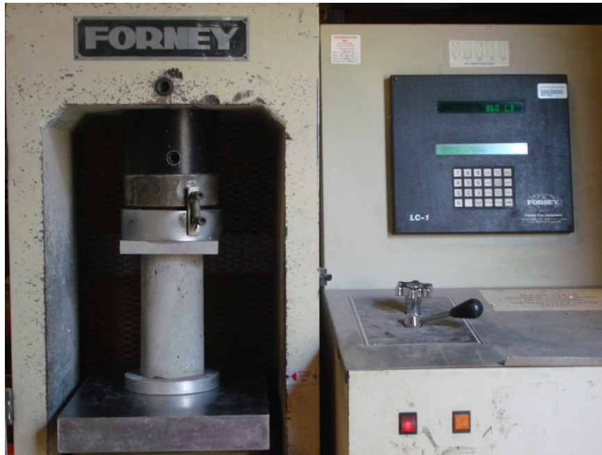
Figure 4.34: Cylinder Specimen Located in Forney Machine Ready for Test
