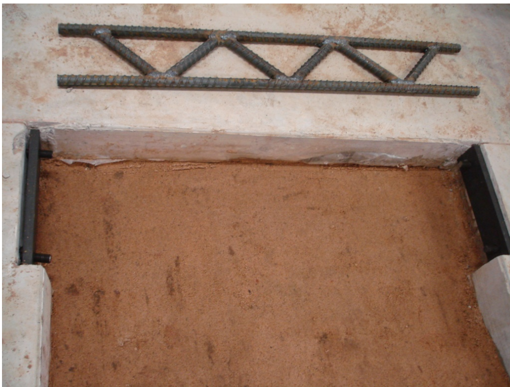
Figure 4.2: End of Slab before Welding Truss to the End Plate
