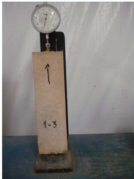
Figure 4.37: Measuring Prism Length Change
