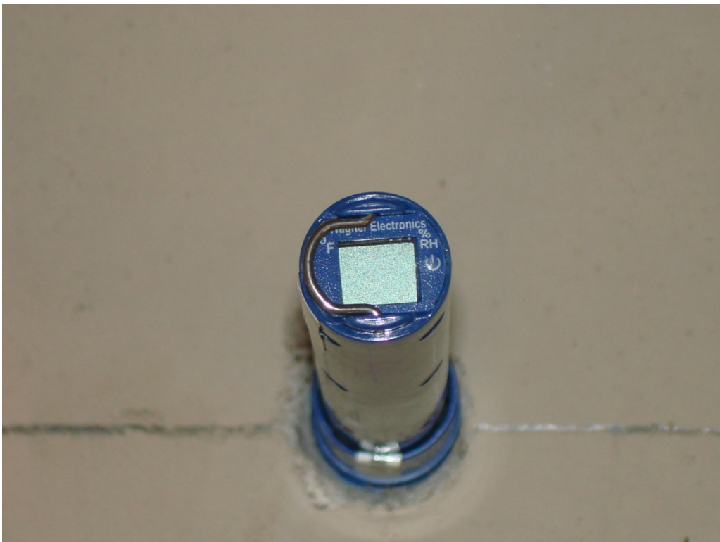
Figure 4.43: Meter for Measuring Interior Slab Temperature and Relative Humidity
