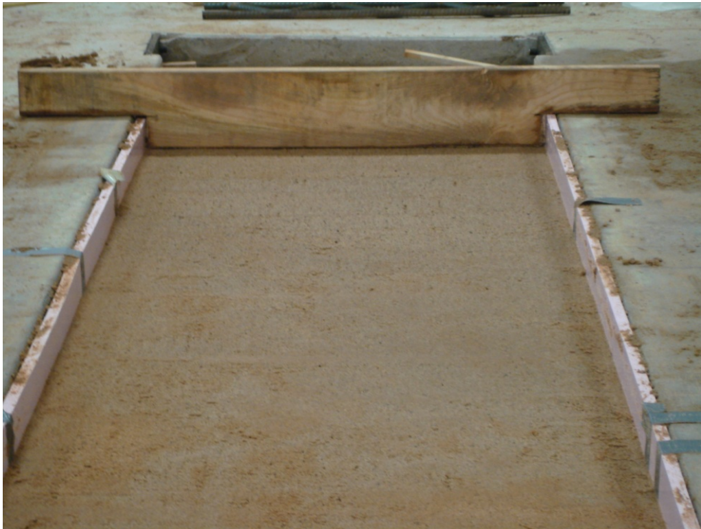
Figure 4.6: Four inches Moist Compacted Sand
