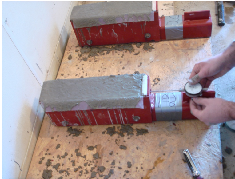
Figure 5.32: Test Frame with Dial indicator strain gage
