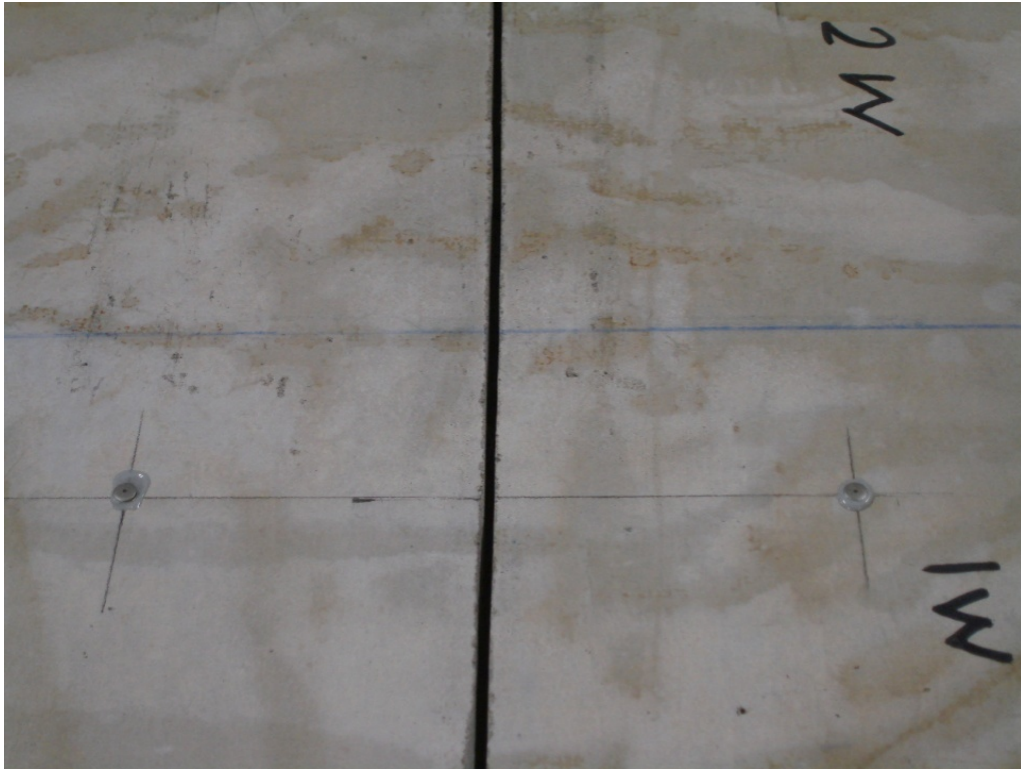
Figure 4.25: Demec Target Located at Saw Cut Contraction Joint
