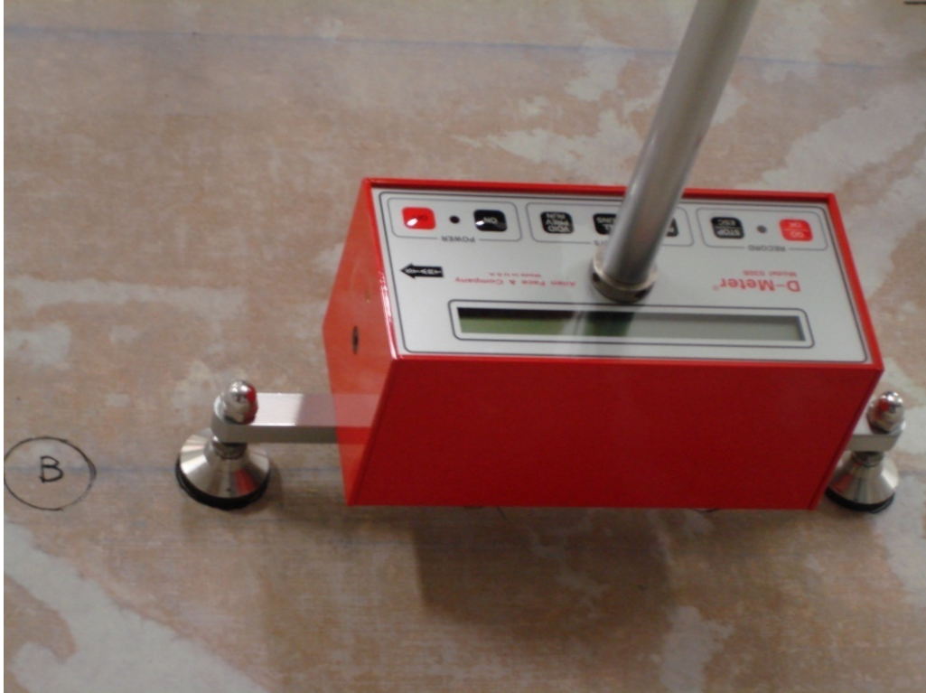
Figure 4.32: Manual Dipstick Device, Measuring Vertical Elevation
