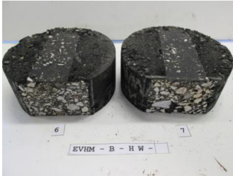
Figure 4.6 EVHM-B Samples after Hamburg Wheel Tracking Test
