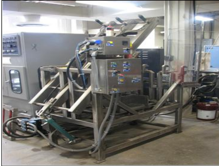
Figure 3.24 Linear Kneading Asphalt Compactor used for Compacting Slab Sample
