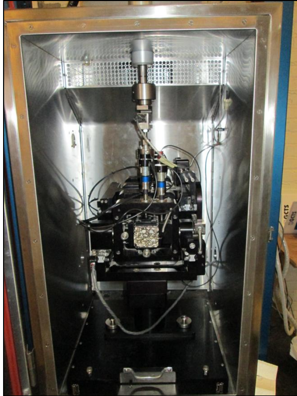
Figure 3.26 Beam Specimen in Fatigue Fixture Inside Temperature Chamber
