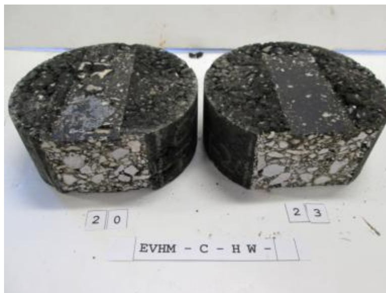
Figure 4.8 EVHM-C Samples after Hamburg Wheel Tracking Test
