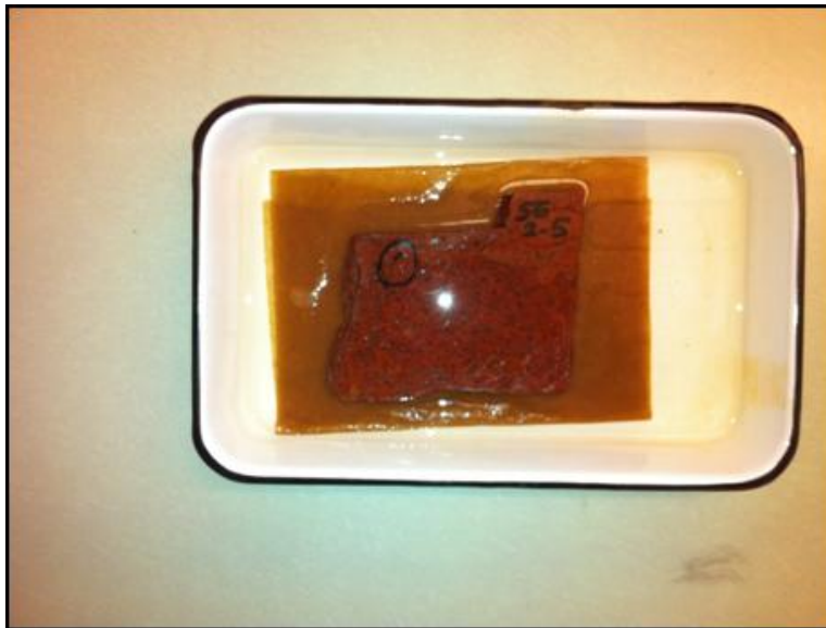
Figure 3.38 Cleaning the Sample with Hexane
