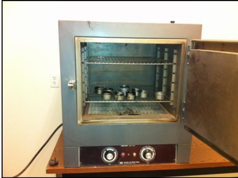
Figure 3.44 PG 64-22 Binder Divided into a Number of Tin Canisters and Kept in the Oven
