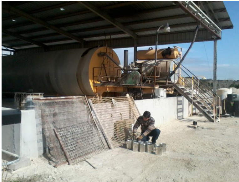
Figure 3.19 Collection of Asphalt Binder from Century Co. Asphalt Plant Located in San Antonio, TX
