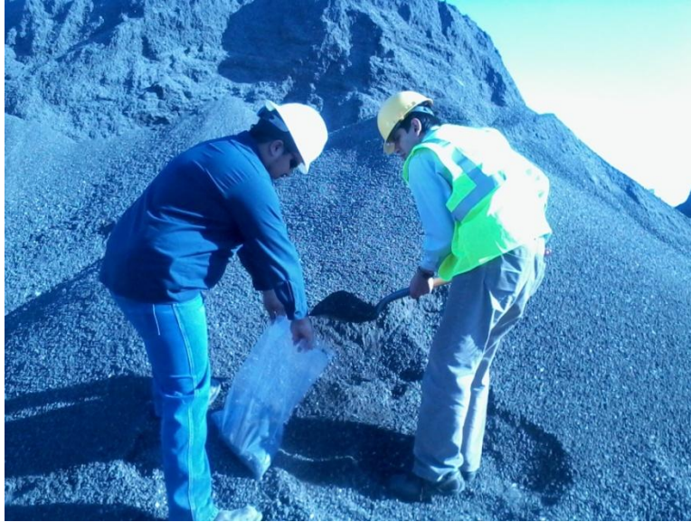
Figure 3.11 Aggregate Collection from Asphalt Plant, San Antonio, TX
