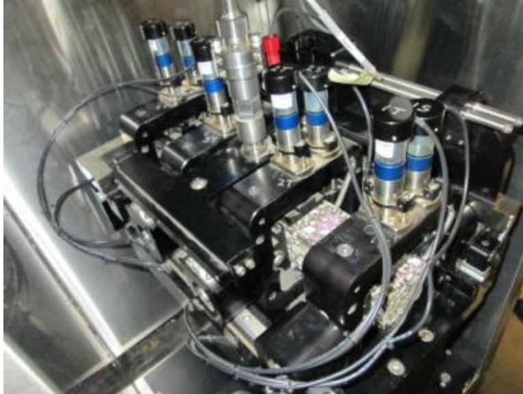
Figure 4.14 Beam Sample in the Fatigue Fixture being Tested inside the Environmental Chamber
