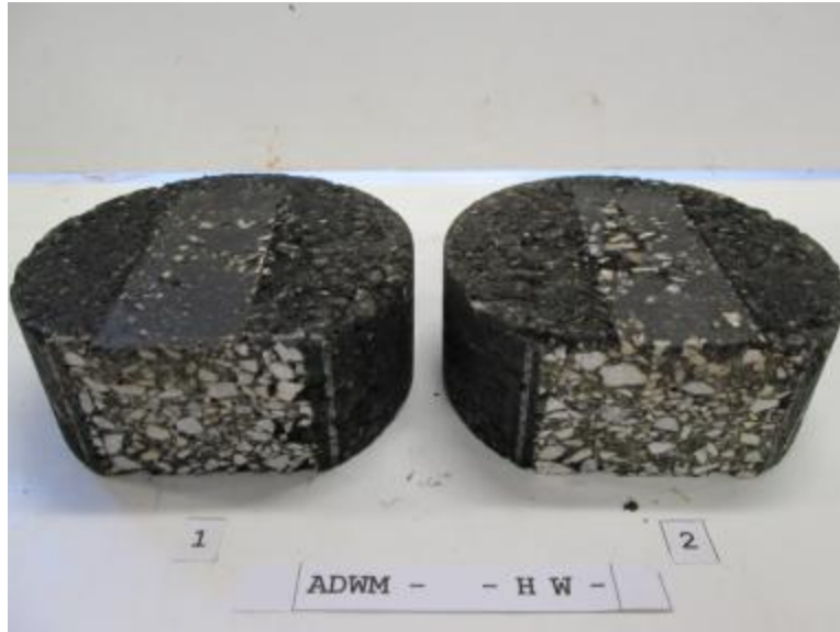
Figure 4.5 ADWM Samples after Hamburg Wheel Tracking Test
