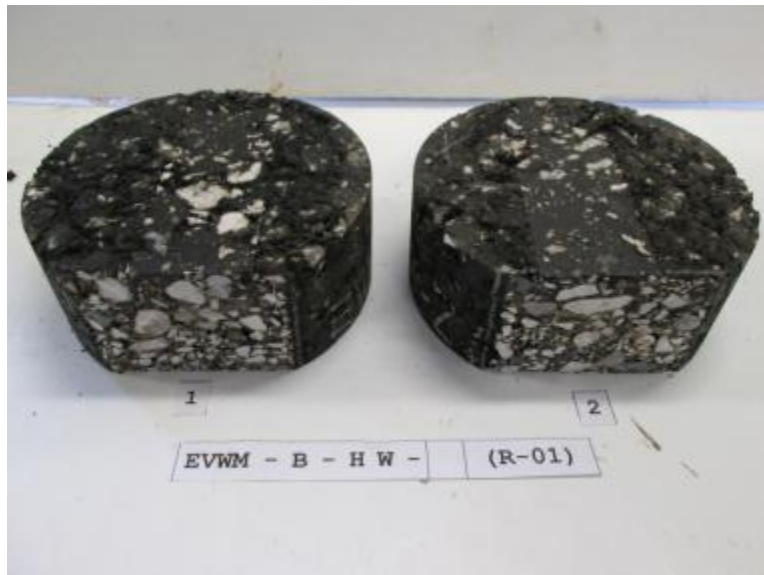
Figure 4.7 EVWM-B Samples after Hamburg Wheel Tracking Test
