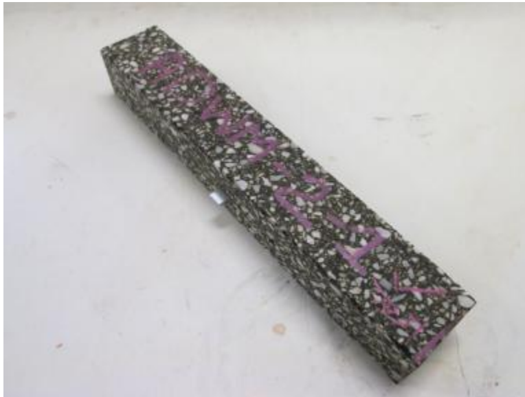
Figure 4.13 Asphalt Beam Specimen with Installed Metallic LVDT Stud
