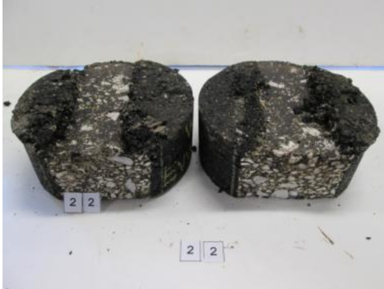
Figure 4.9 EVWM-C Samples after Hamburg Wheel Tracking Test
