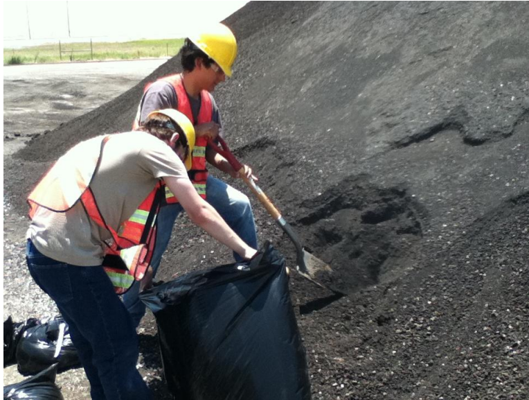
Figure 3.5 RAP Collection from Asphalt Plant in Bridgeport, TX
