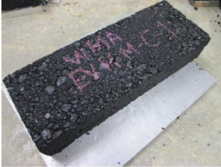
Figure 4.12 Compacted Slab using a Kneading Compactor
