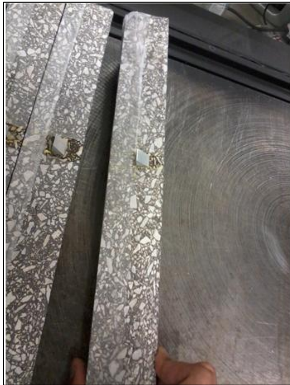
Figure 3.25 Four-Point Bending Beam Fatigue Specimen with the Metallic Target Mounted
