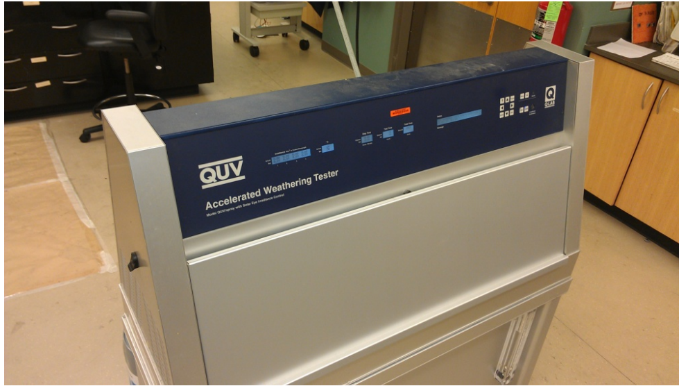
Figure 4.3: Test chamber used for alternating exposure of UV and condensation
