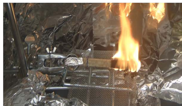
Figure 4.4: Test setup for determining flame propagation rate
