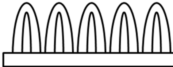
Figure 2.4 Loop - pile type carpet (when the loops are cut, it remains uncut) [16]
