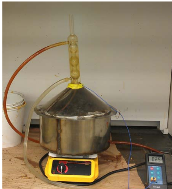
Figure 4.2: Moisture absorption test set up of carpet composites
