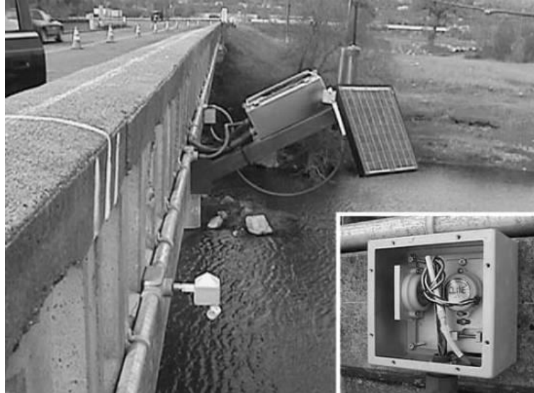
Figure 2.11. Tilt sensor installation with detail of the sensor (cited by Hunter 2009).
