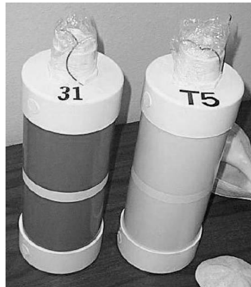
Figure 2.9. Float-out devices color coded and numbered for identification (Texas Transportation Institute, cited by Hunter 2009).
