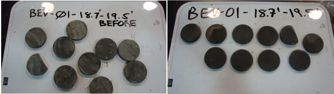
Figure 2 – Example of rock samples before (left) and after (right) continuous slake durability testing.
