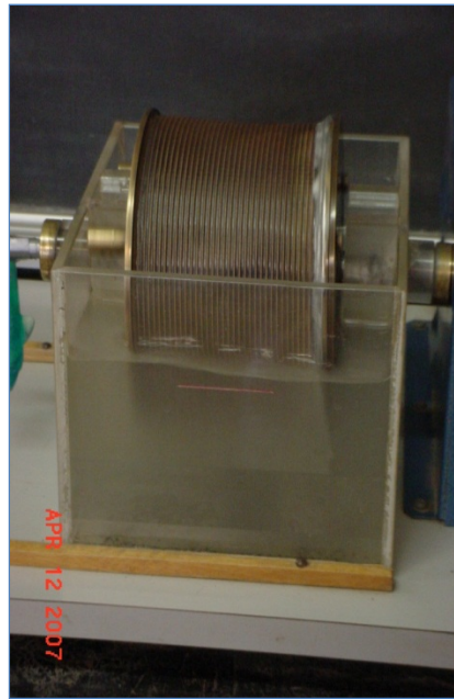
Figure 1 – Rotating drum used in the continuous slake durability tests.
