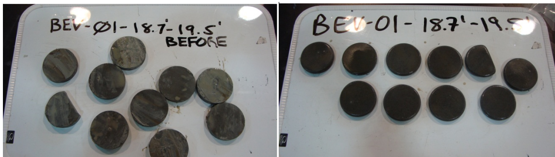
Figure 13 – Example of rock samples before (left) and after (right) continuous slake durability testing.
