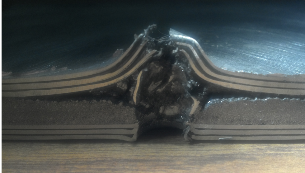
Figure 10. Image of TCON A sandwich composite after absorbing 252 J of energy.
