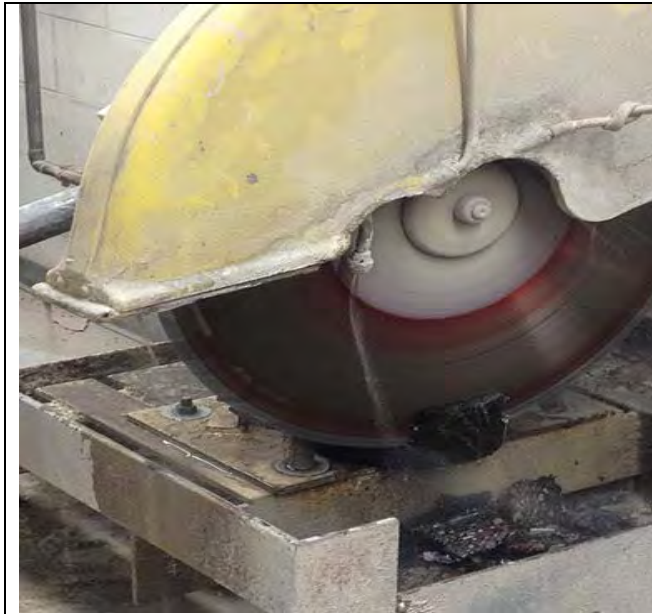
(a) Specimen being cut along edge of the mold using masonry saw
