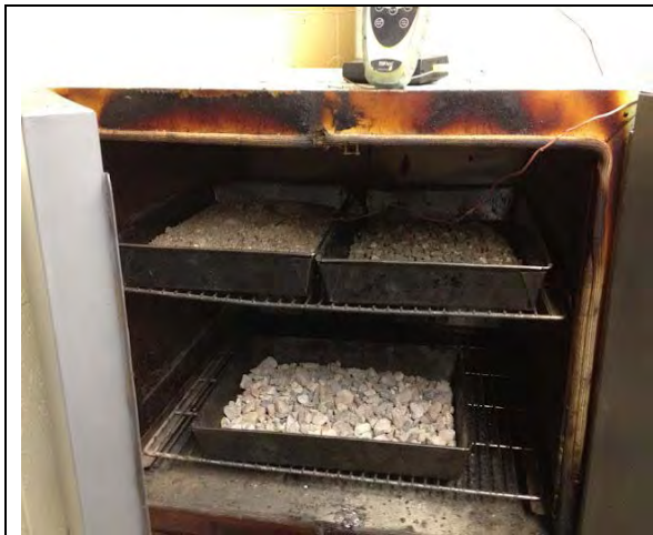
(a) Heating aggregate to mixing temperature in oven
