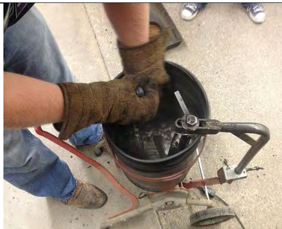
(c) Mixing of asphalt and aggregate in the mixer
