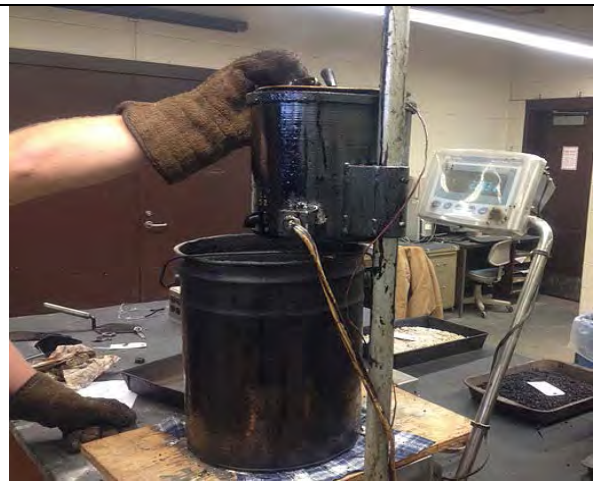
(b) Adding asphalt to the aggregate in the mixer
