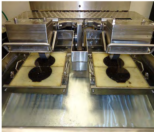
(c) Specimens placed in molds and mounted in tray, ready for testing
