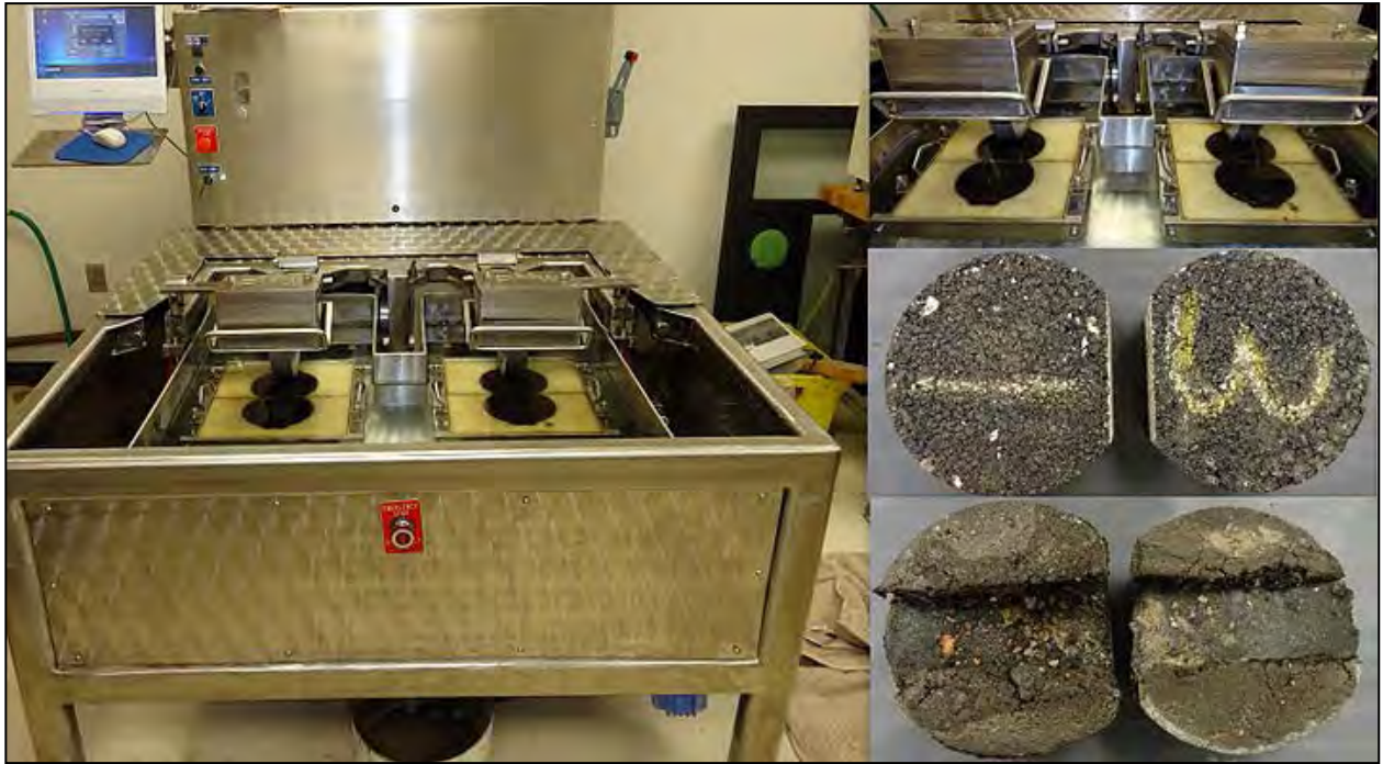
FIGURE 2.1 (Clockwise) Final Test Setup of Hamburg Wheel Tracking Device, Close-Up of Specimens under the Wheel Load, Specimens Ready for Testing in HWTD, and Failed Specimens with High Rut Depth
