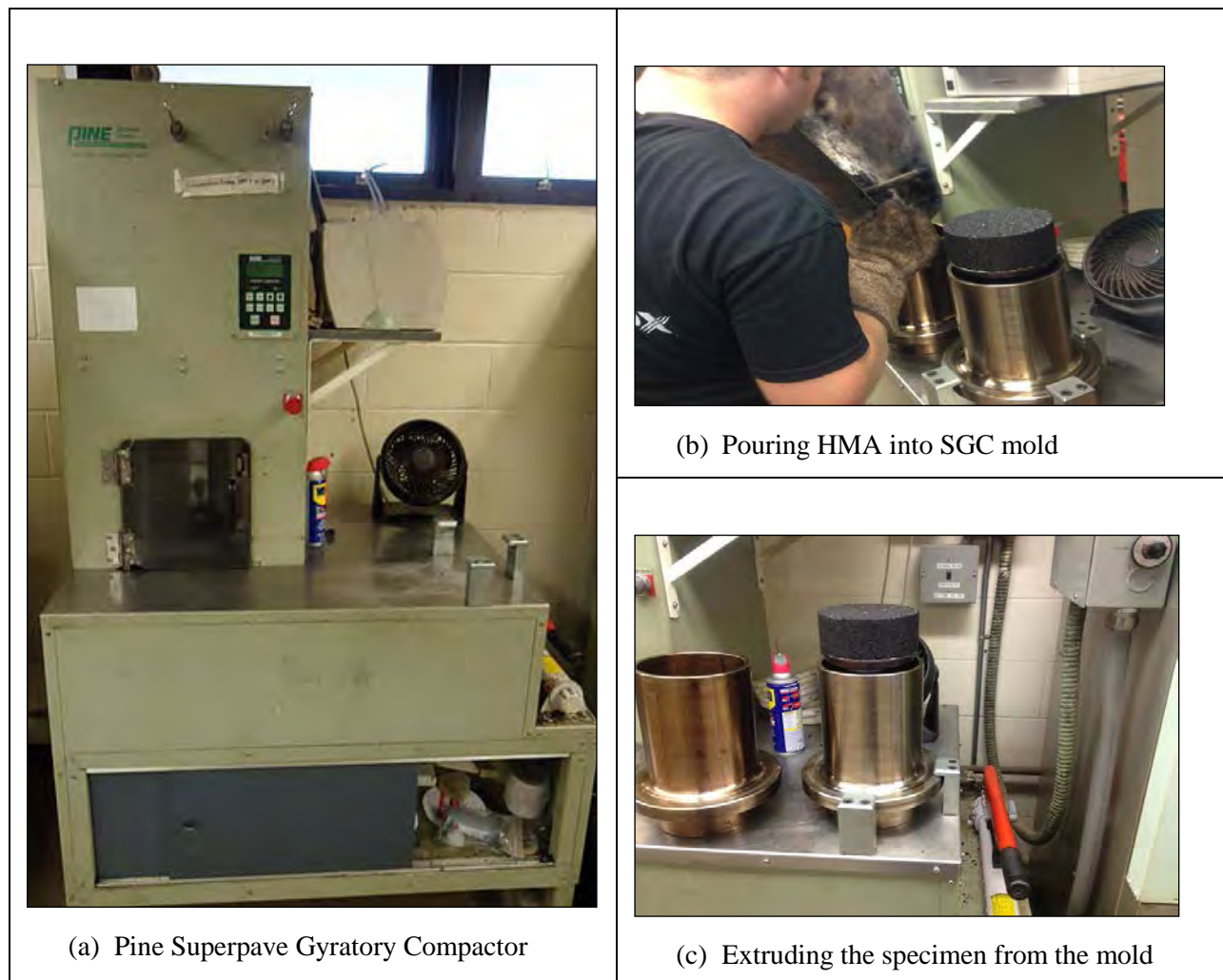
FIGURE 3.2 Compacting Specimen Using Superpave Gyrotory Compactor
