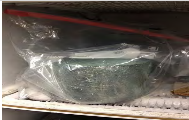
(c) Specimen freezing @ -18°C for at least 16 hours
