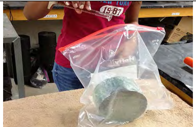
(b) Specimen wrapped with plastic film enclosed in heavy-duty, leak-proof bag with 10 ml of water
