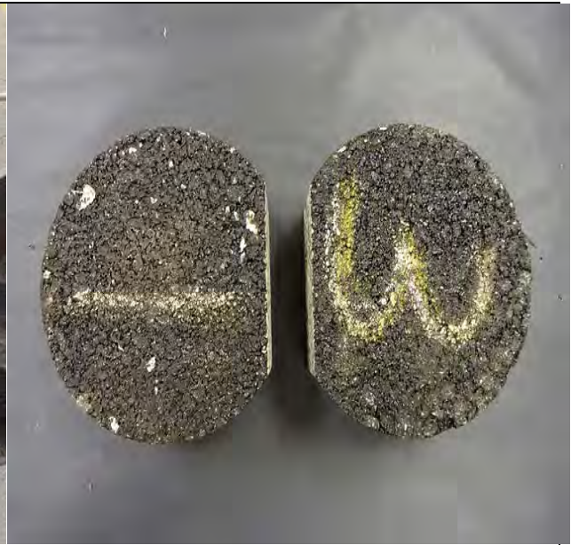
(b) Vertical-cut specimens (approx. 5/8 inch)
