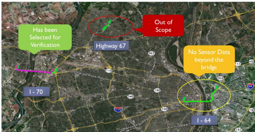
Figure 3-3: Bluetooth-based travel time data collection sites. The background image is from Google Earth.
