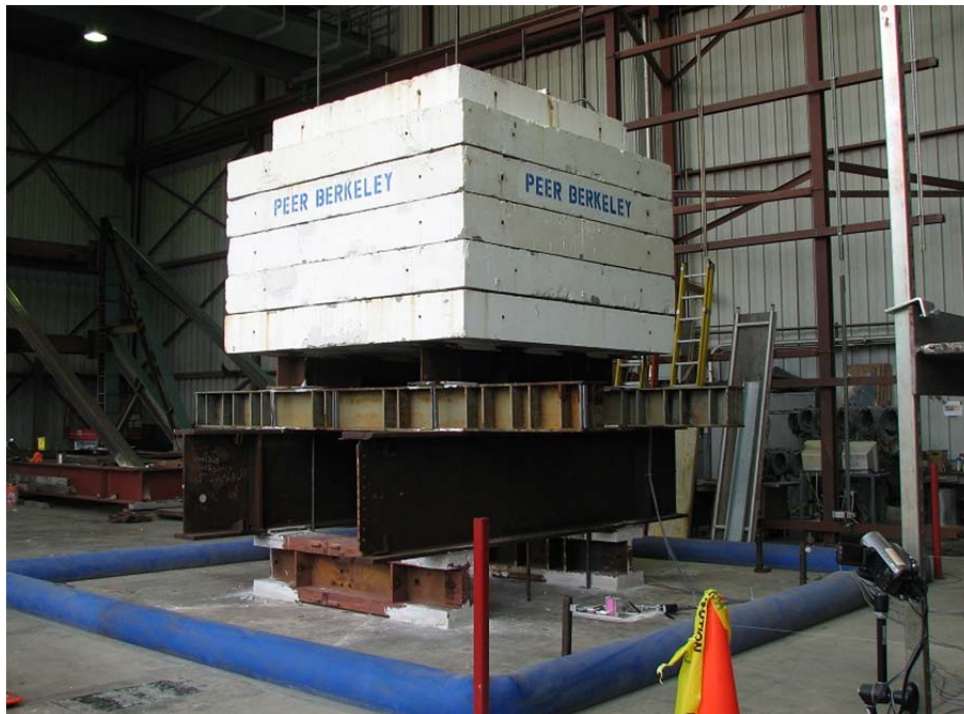
Figure 3-2: Photograph of the fidelity test setup
