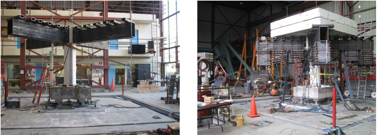
Figure 4-2: Photographs of the pullback tests without (left) and with (right) total mass
