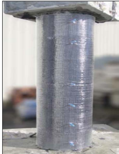
GFRP repaired SP1
