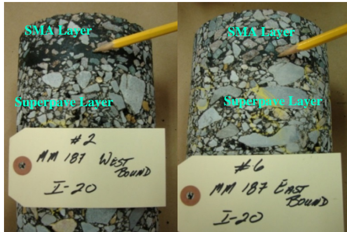
Figure 40 Aggregate arrangement in the SMA mixture
