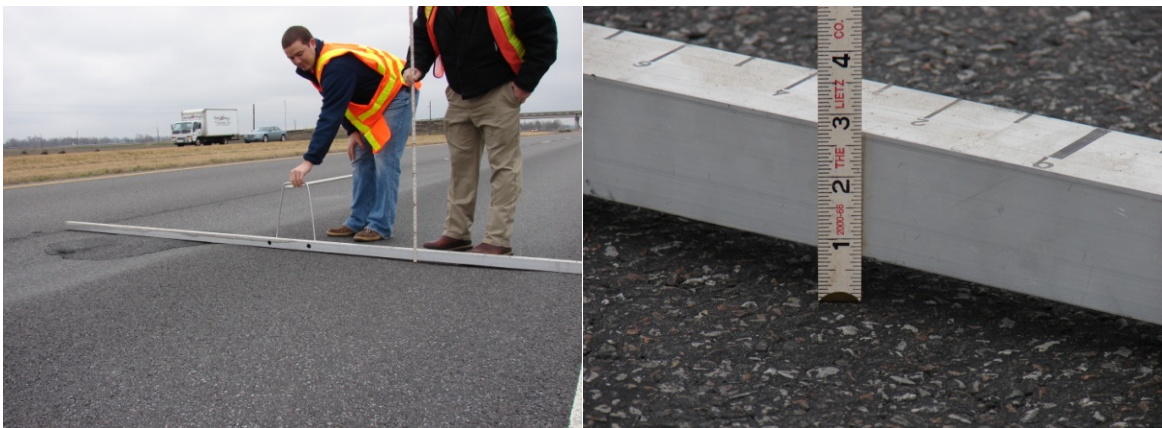
Figure 2 Localized rut measurement using traditional straight edge
