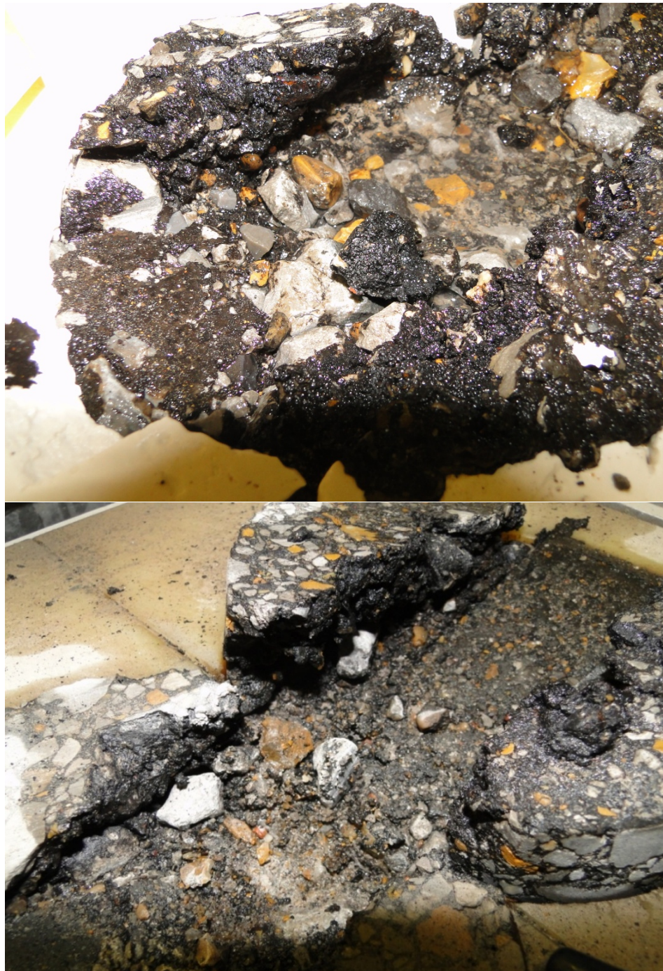
Figure 32 Moisture damage observed on cores after LWT test
