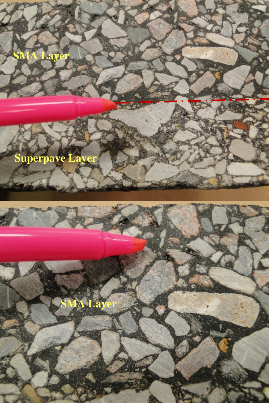
Figure 35 Aggregate arrangements in the SMA mixture
