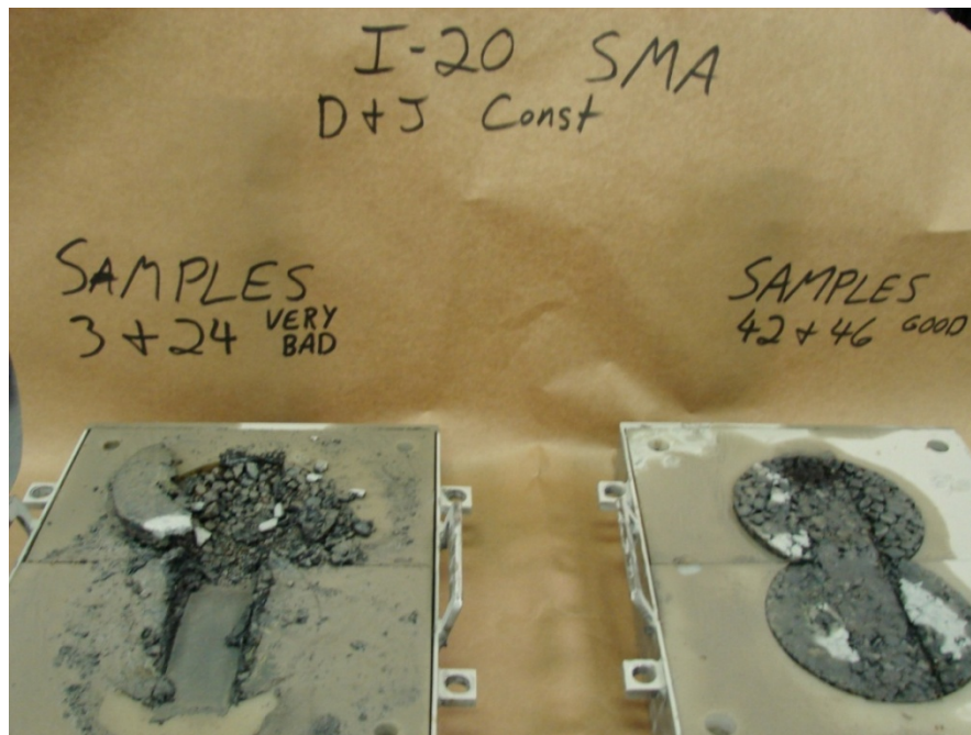
Figure 37 Roadway Core from Very Bad Section after LWT Test
