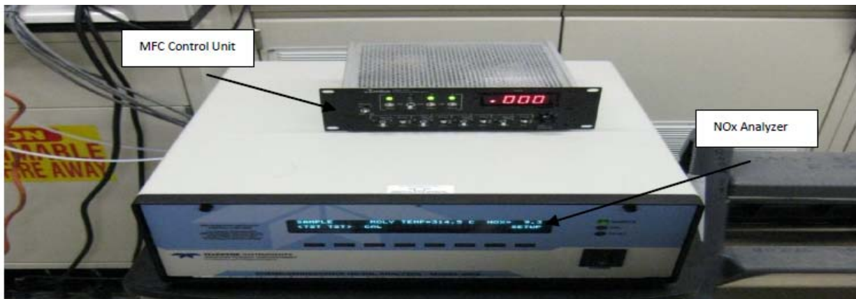
Figure 2. Experimental setup developed in our lab to evaluate the efficiency of coatings for removal of NO 2 , a priority air pollutant.
