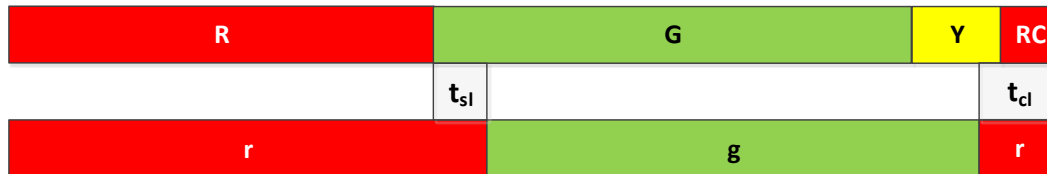
Figure 37. Relationship between displayed green time, effective green time, and lost time
