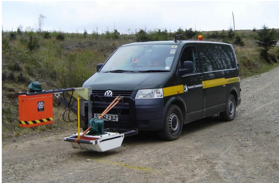
Figure 33. Air borne GPR survey vehicle used for condition assessment on ROADDEX projects in Europe (Drake 2012)
