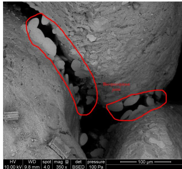
Figure 24. SEM image from bio-treatment of silica sands at ISU (350x) (Li, 2012)
