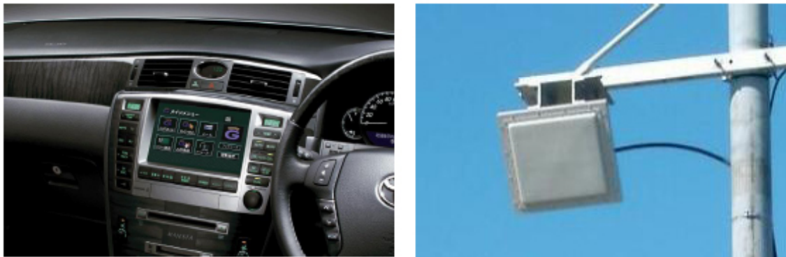
Figure 5-13. An ITS Spot-compatible car navigation system (left) and ITS Spot roadside equipment (right) (Source: MLIT)[43]
