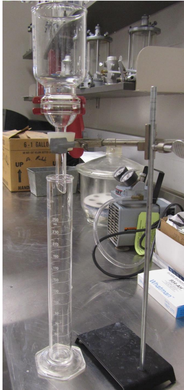
Figure 4.6 Filtration system with no vacuum
