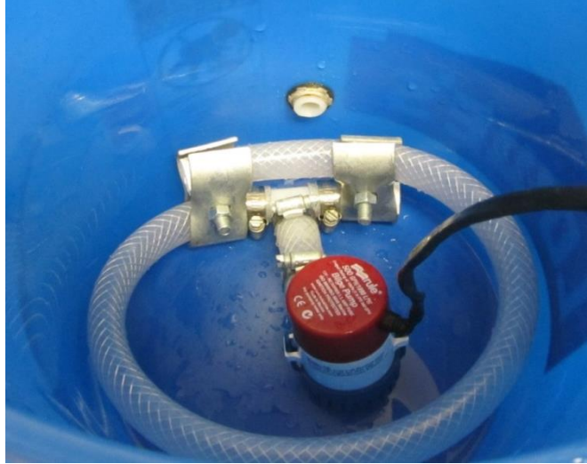
Figure 4.1 Bilge pump mixing apparatus used for keeping particles in suspension
