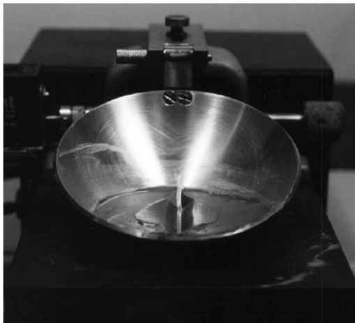
FIG. 7 Grooved Soil Pat in Liquid Limit Device
