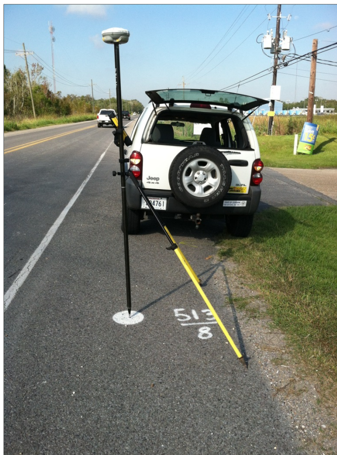
Figure 3 GPS equipment installed at a control point (#513) along the west-bound shoulder of Hwy 70
