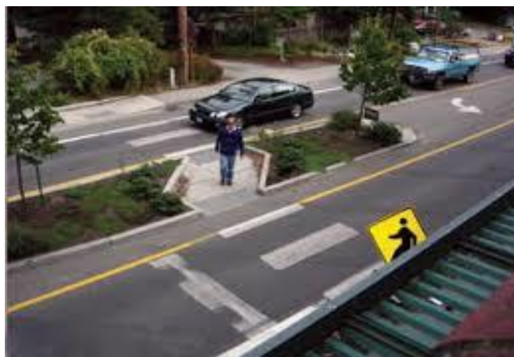
Figure 2-9: Pedestrian Refuge Island (FHWA, 2013)
