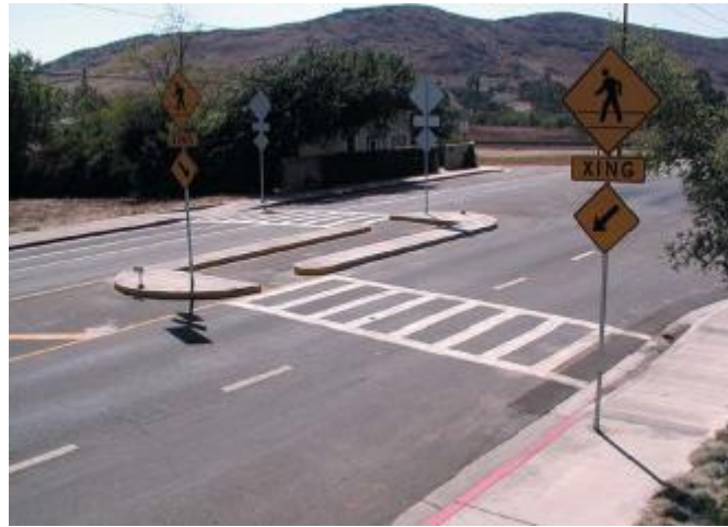
Figure 2-6: Crosswalk with Ladder Pattern (Harkey and Zegeer, 2004)
