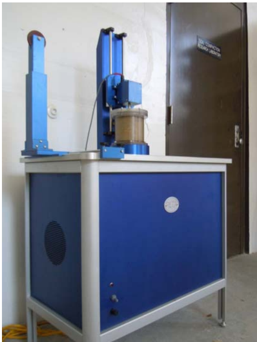
Figure 2-8. The rotating erosion testing apparatus
