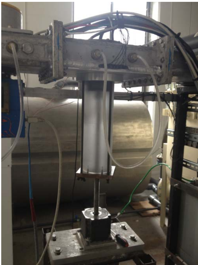
Figure 3-8. SERF with new testing tube
