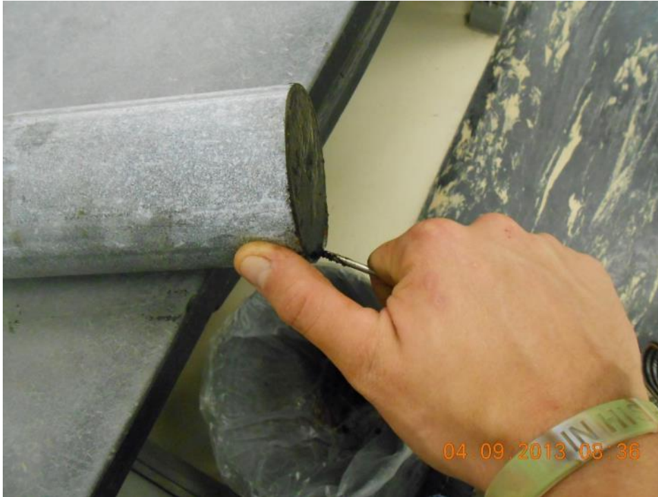
Figure A-33. Removing Shelby tube burs using a file
