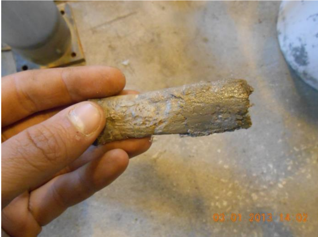
Figure 6-6. More evidence of organic matter responsible for erosion disturbances
