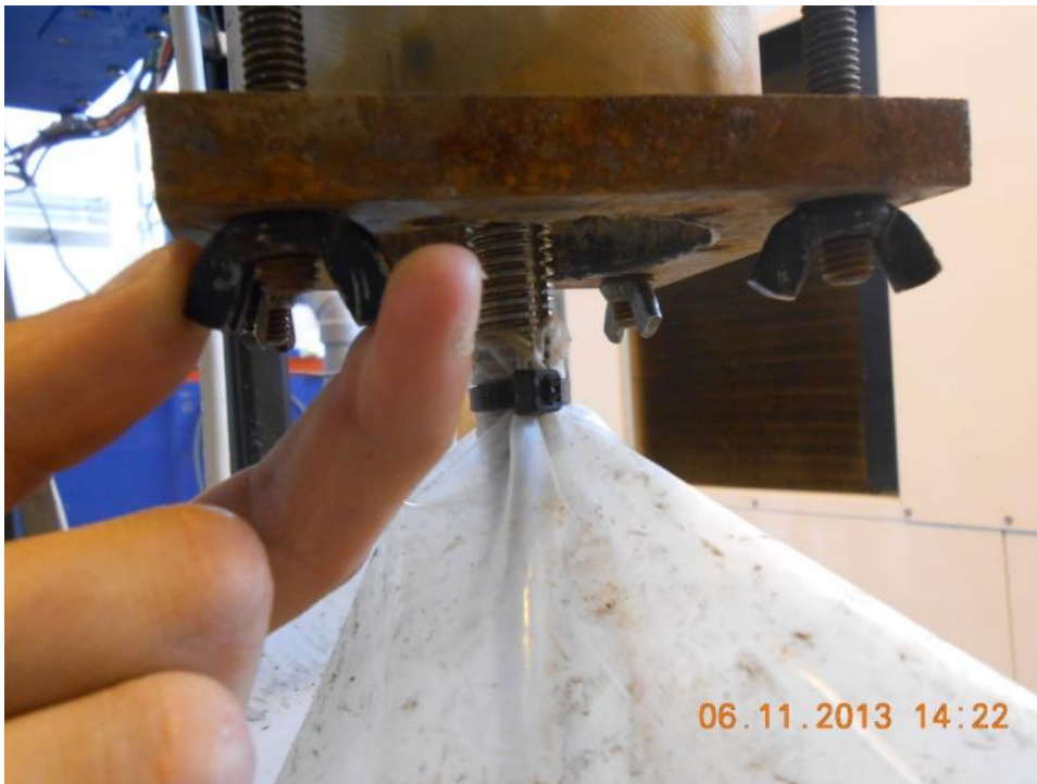
Figure A-40. Attaching wing nuts to SERF compression plate
