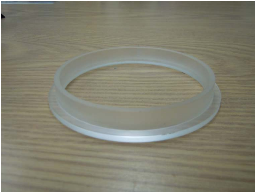
Figure 3-2. Plexiglas insert for use in the laser system
