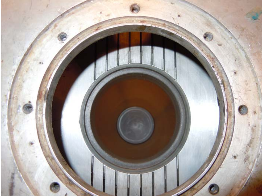
Figure A-17. Top-view into SERF (SEATEK removed) showing laser and photoelectric sensor grooves
