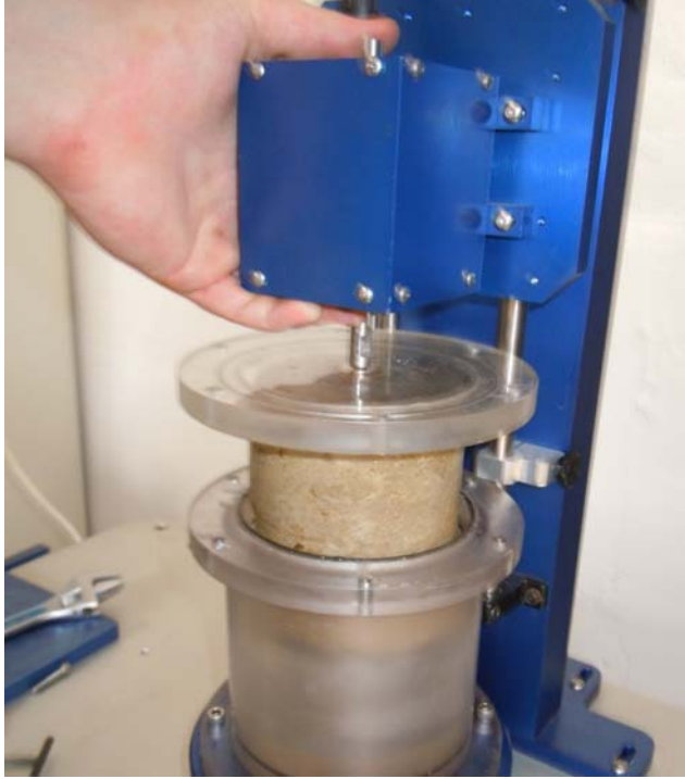
Figure 2-13. Lowering the RETA sample into position
