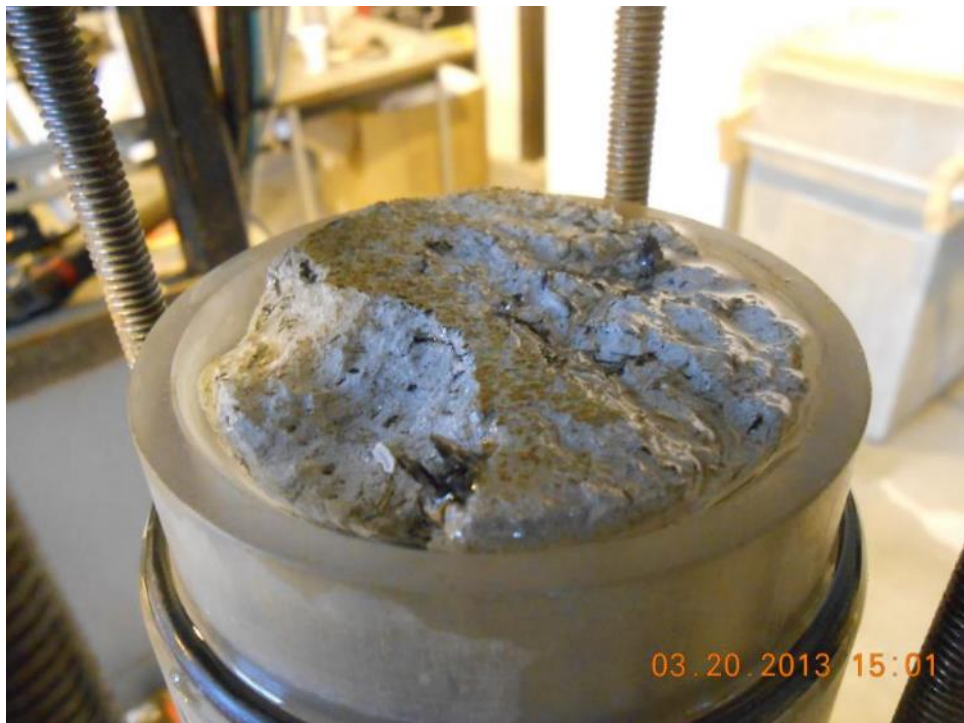
Figure 6-8. Photograph of JCB 10'-12', dry, test 1 after application of approximately 5 hours of very high shear stresses
