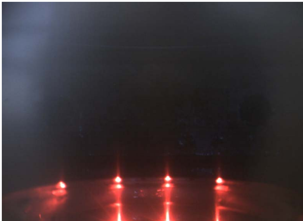
Figure A-8. Photograph inside SERF showing lasers (note 4 laser point one direction and 4 lasers point another direction to minimize interference)
