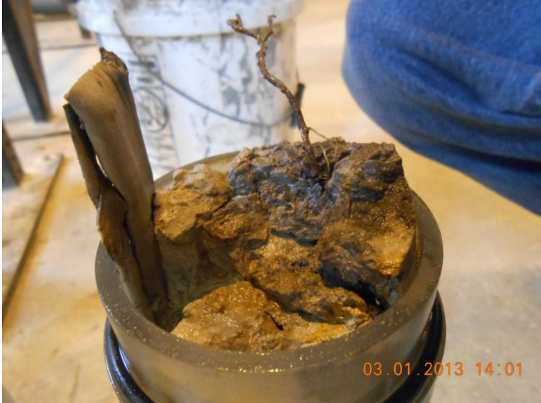
Figure 6-5. Evidence of organic matter obstructing erosion
