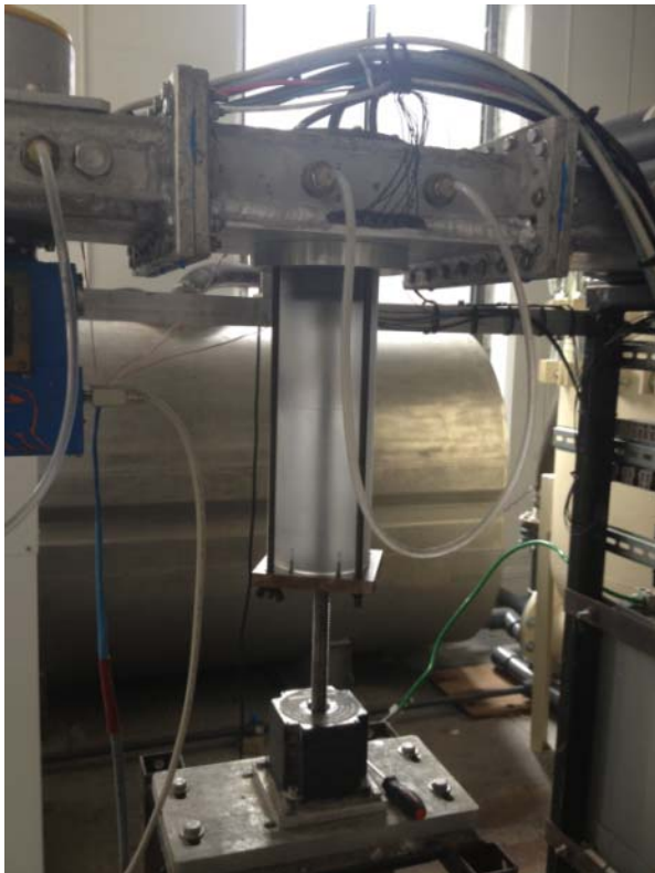
Figure A-16. SERF close-up showing the compression plate
