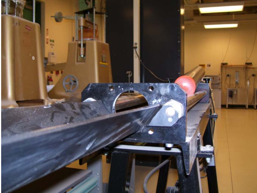
Figure A-5. FDOT Shelby tube extractor to be used with SERF test tubes
