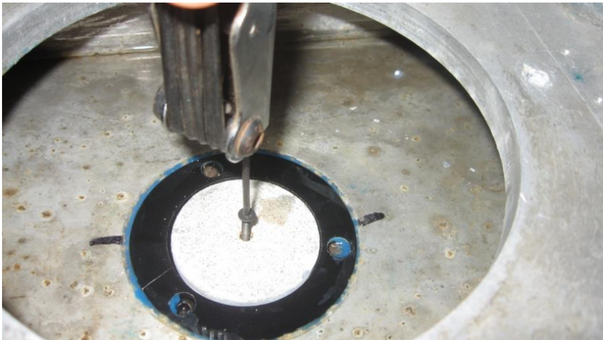
Figure A-24. Illustration of affixing a test-disc to the shear stress sensor
