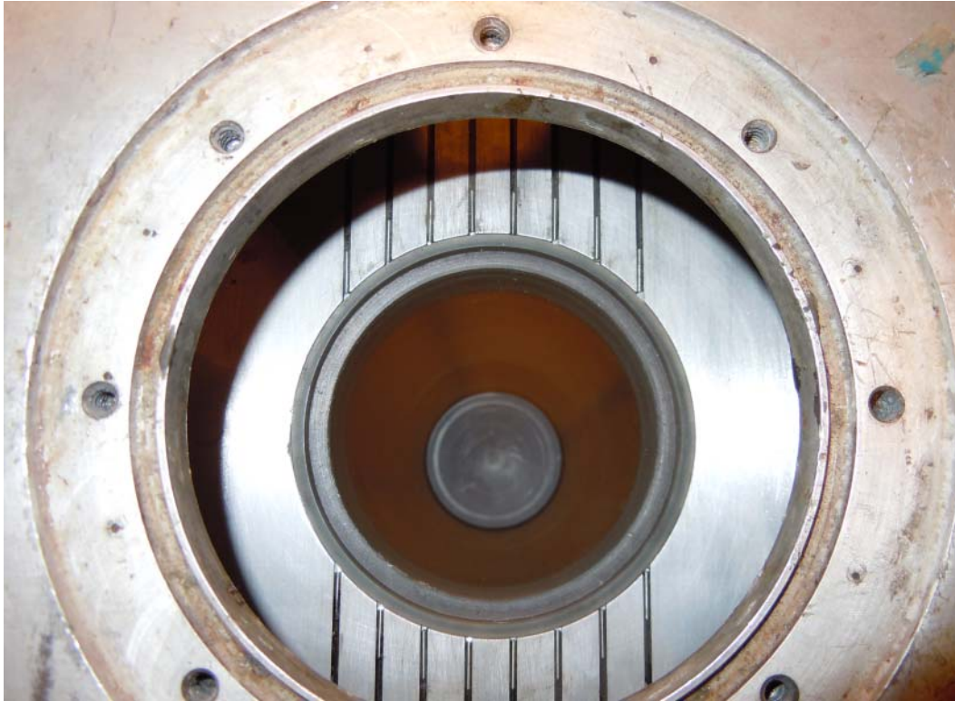
Figure 3-1. New laser bank (top looking down into sample tube). Please note that lasers/photoelectric sensors have been set up to alternate
