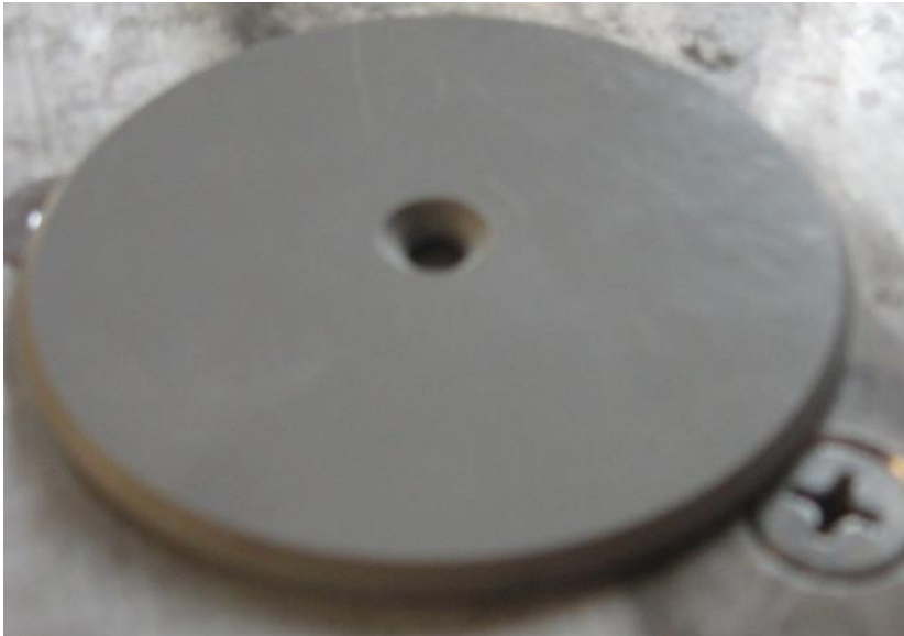
Figure A-20. Example of shear stress sensor removable test-disc
