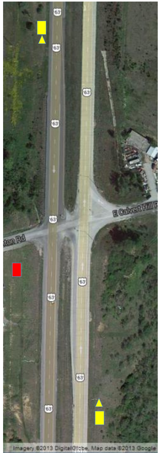
Figure 3.9 Location of cameras, radars, and delineators at the control site
