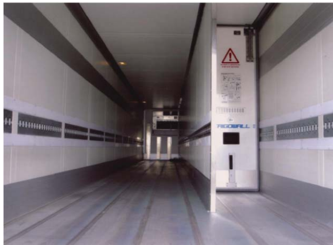
Figure 1 Aluminum Floor (Source: Goevaers, R., 2010)
