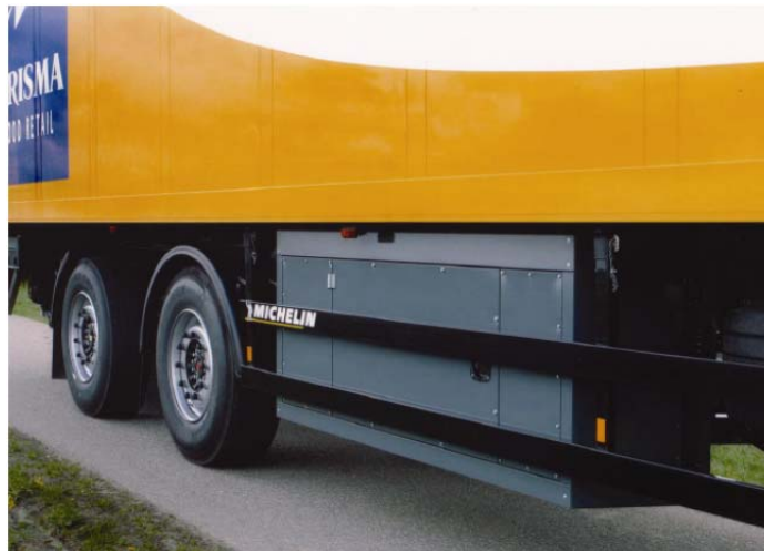
Figure 2 Refrigeration Unit (Source: Goevaers, R., 2010)
